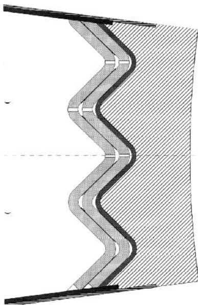
Concerning the toroïdal field coils, the use of mineral insulators would authorize the decrease of the thickness of the shielding, on the high field side, to a value of 0.2 to 0.3 m. In view of the high level of irradiation, no impregnation under vacuum with resins would be envisaged. Moreover, the coils would not be cooled by water but by organic fluids.
