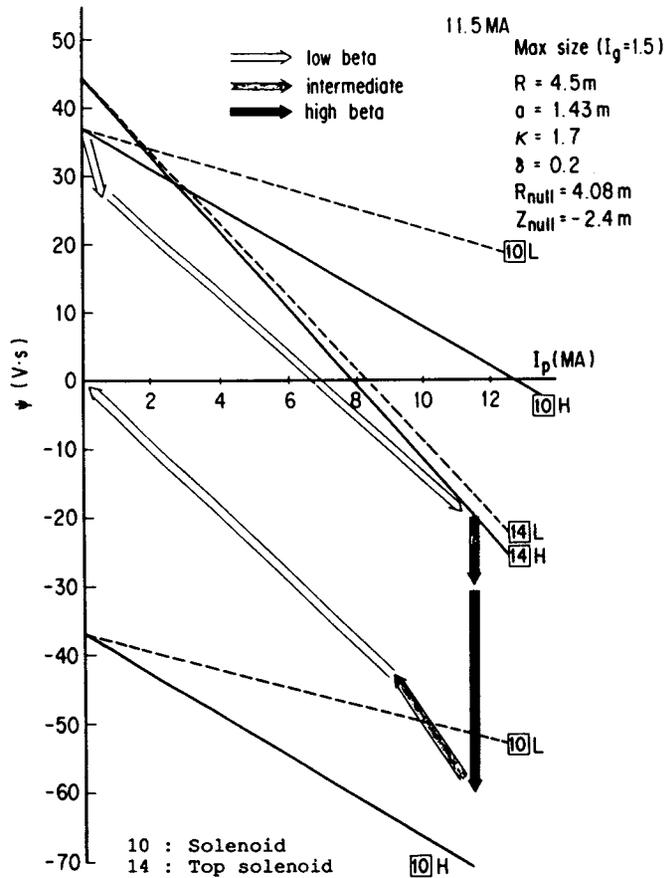
FIG. 2. Operation space in the plane of supplied flux,  $\psi$ , and plasma current,  $I_p$ . Solid and dotted lines are limiting lines for designed operation condition in high and low beta states for each coil, respectively.
