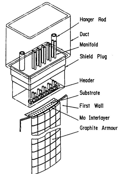
FIG. 3. Guard limiter concept to protect the first wall, which is an easily replaceable 'sacrificial' limiter.
