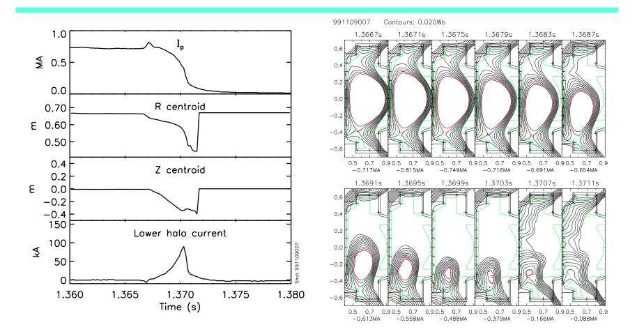
• Plasma starts falling immediately after thermal quench.
