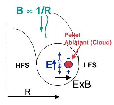
Polarization of the ablatant occurs from ∇B and curvature drift in the non-uniform tokamak field:
