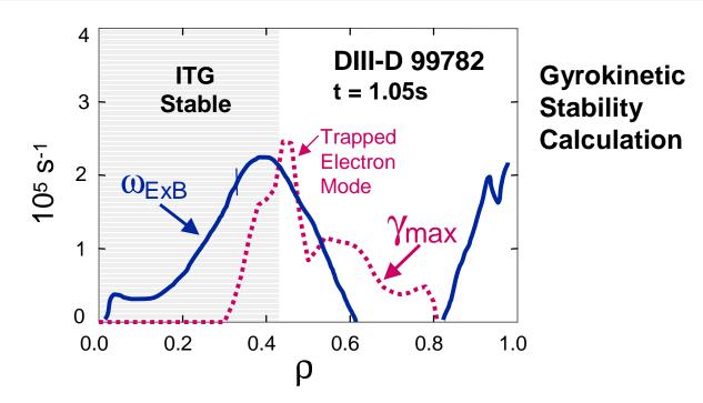
The ExB shearing rate exceeds the ITG growth rate inside the ITB
