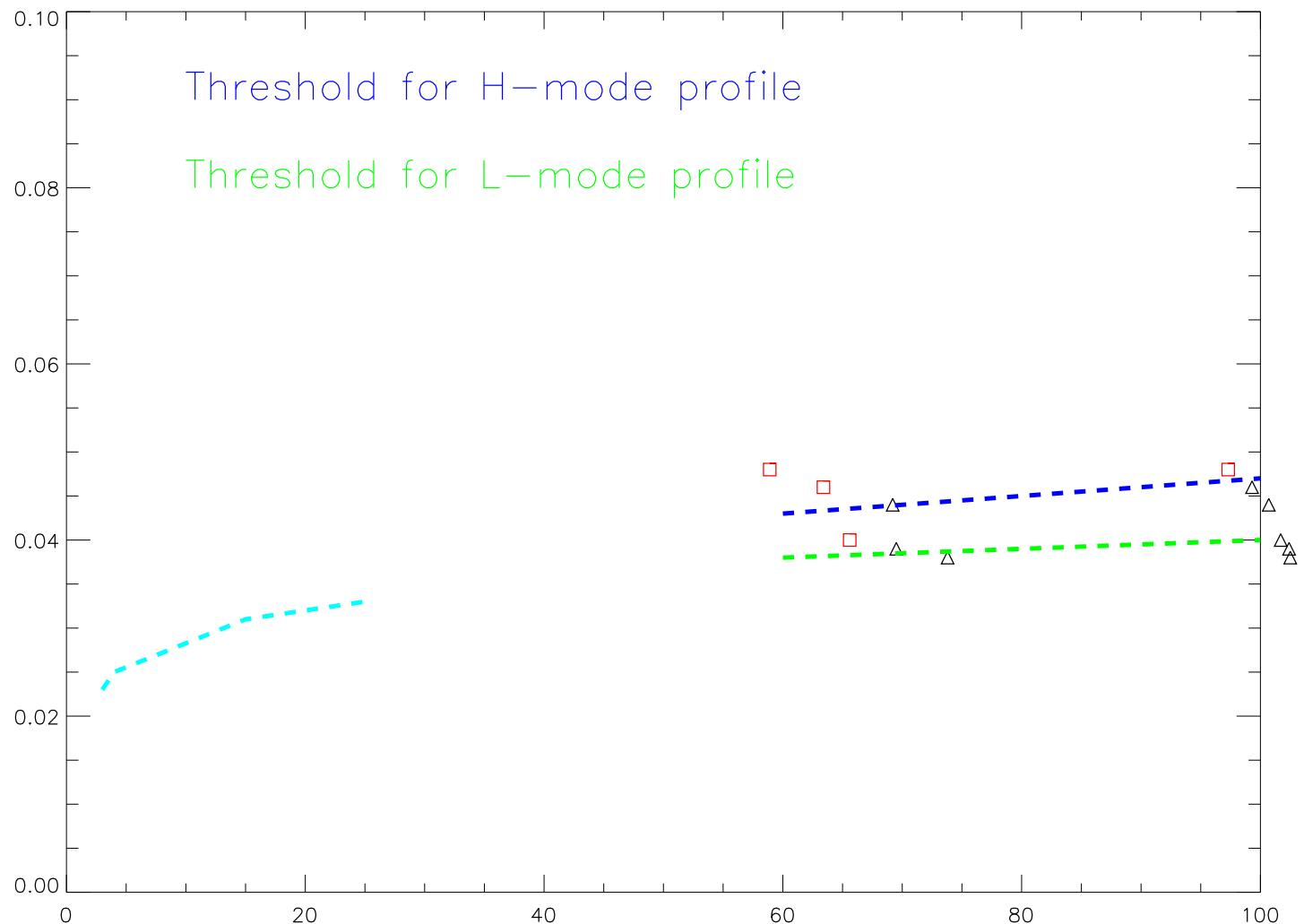
NSTX stability threshold with  $q_{\text{edge}} = 5.5$
