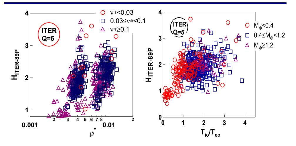
• Higher confinement factor should be obtained at  $T_{i}/T_{e}\sim\!\!1$
