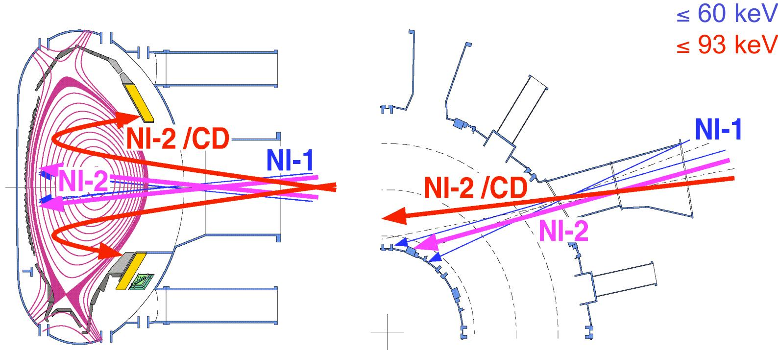
Re-direction of neutral beam injection system
