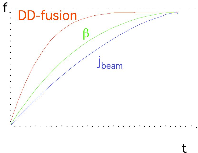
fractional contribution  $f$  of fast particles to DD-fusion,  $\beta$ , and beam current during first  $t$  seconds of their slowing down history
