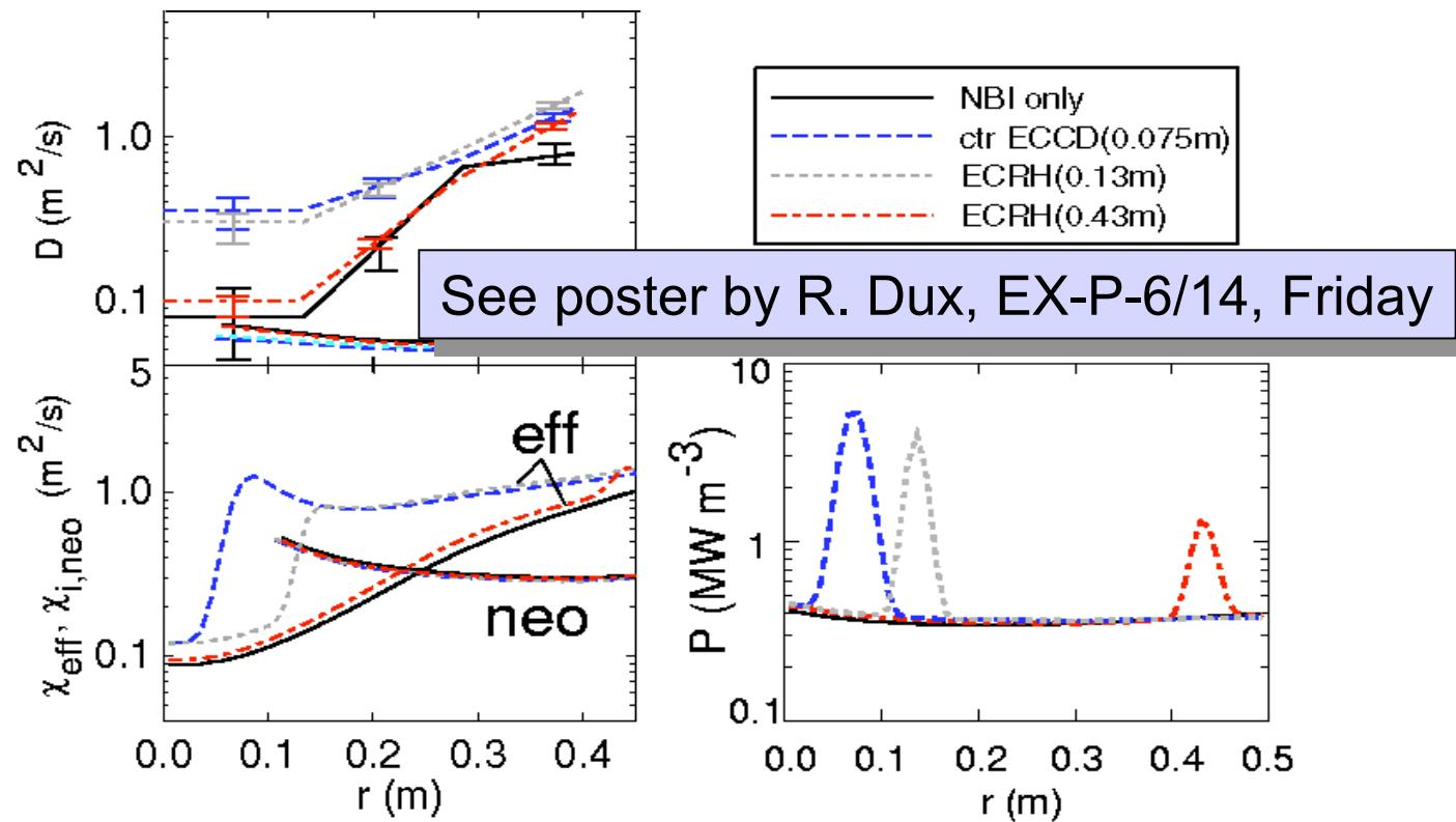
Effect of central heating on density peaking (neoclassical inward pinch) and on anomalous particle transport
