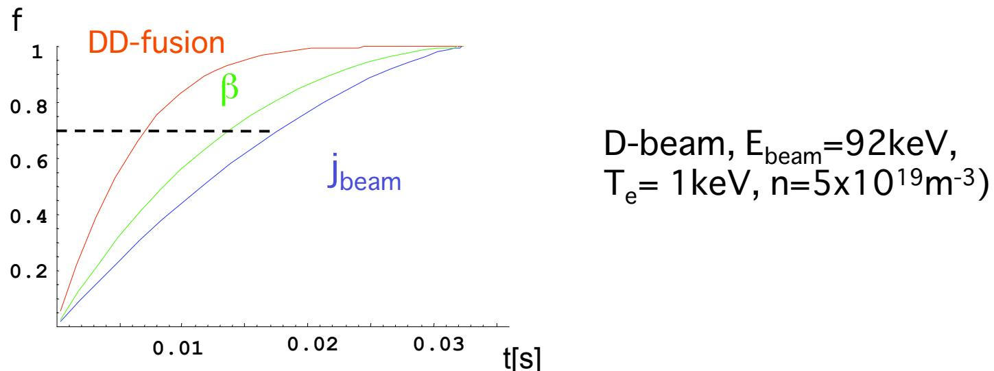
beam current particularly susceptible to diffusion: slowing down particles contribute substantially **longer** to beam current than to energy density or fusion rate
