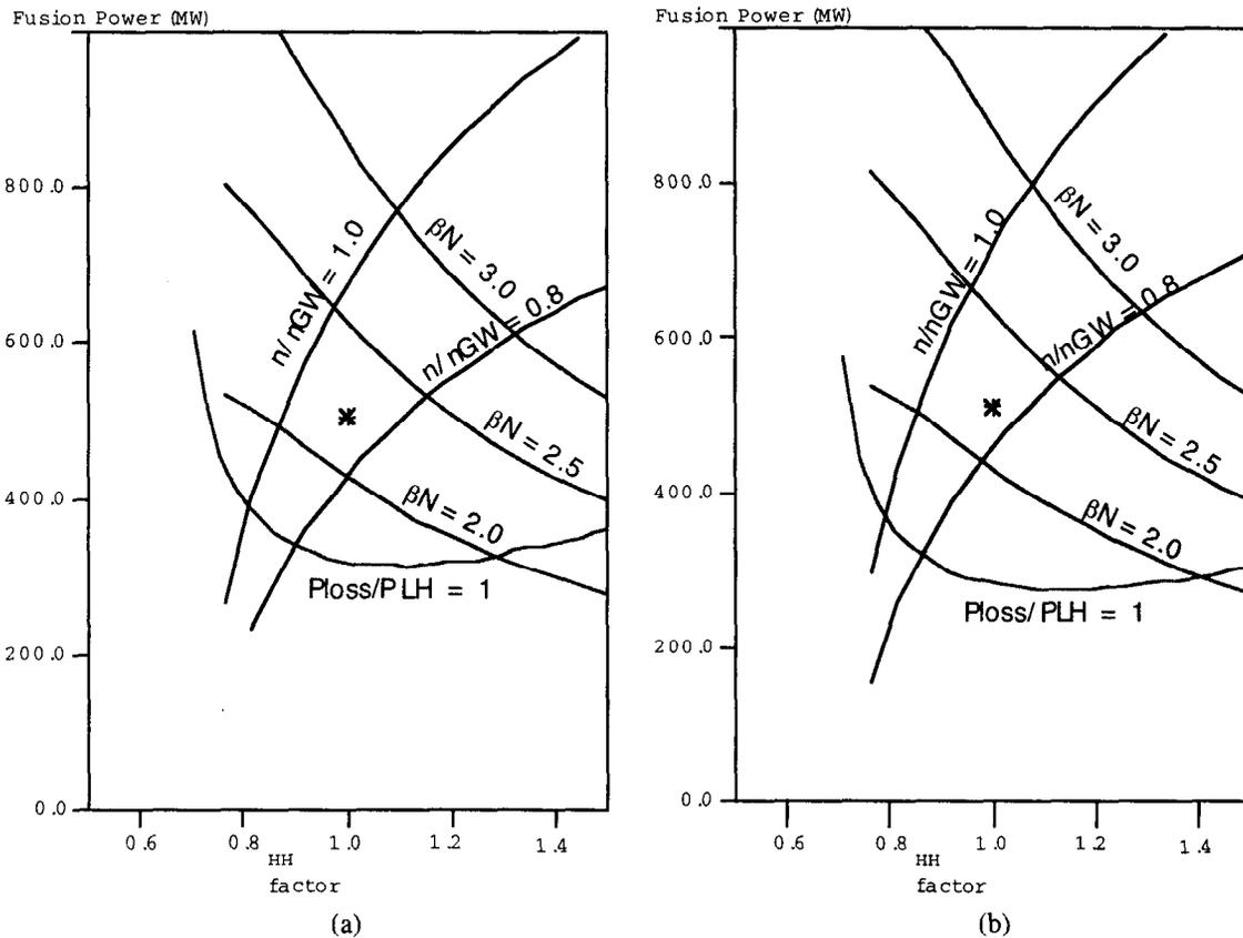
Fig. 5. The  $Q = 10$  operation domain of (a) IAM and (b) LAM.
