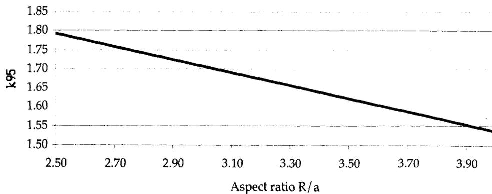
Fig. 2. Dependence of  $k_{95}$  versus plasma aspect ratio used in the system code for aspect ratio scans.
