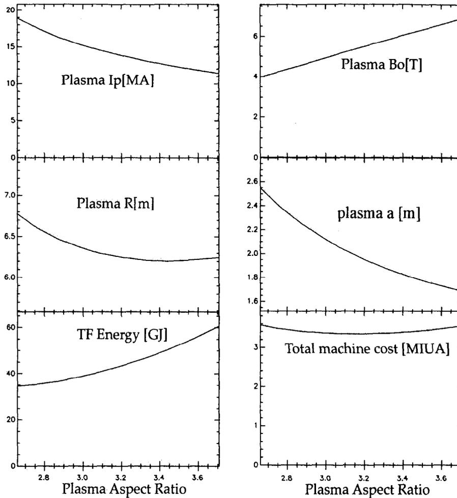
Fig. 3. Variation of some tokamak parameters as a function of aspect ratio.
