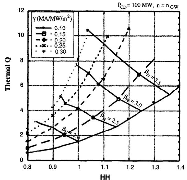
Fig. 8. Effect of CD efficiency on the  $Q = 5$  operation domain.
