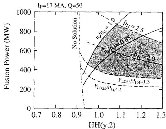
Fig. 16. The  $Q = 50$  operation domain (zero-dimensional modeling) with  $I_p = 17$  MA ( $\tau_{He}^*/\tau_E = 5$ , Be = 2%, Ar = 0.12%).
