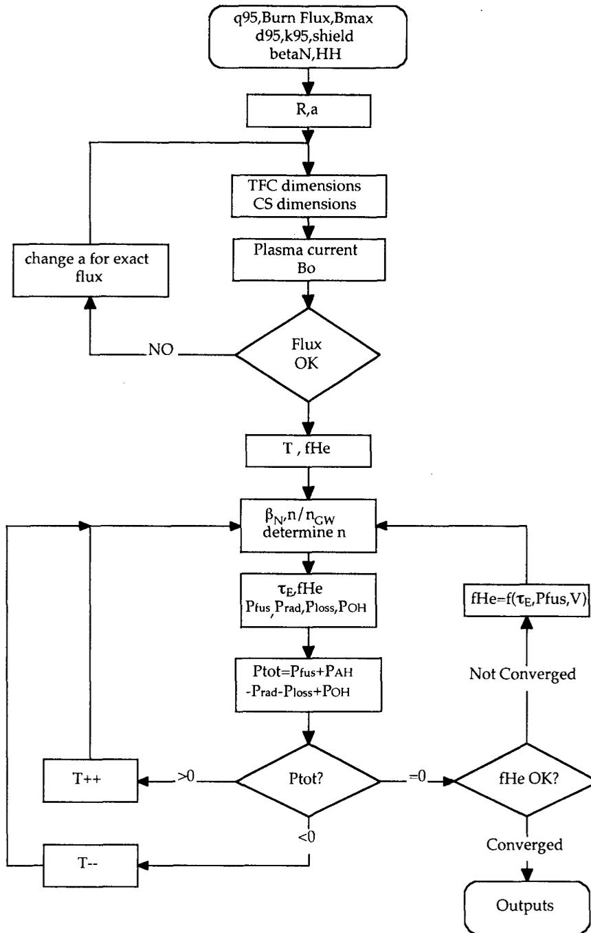
Fig. 1. Flowchart for system code.
