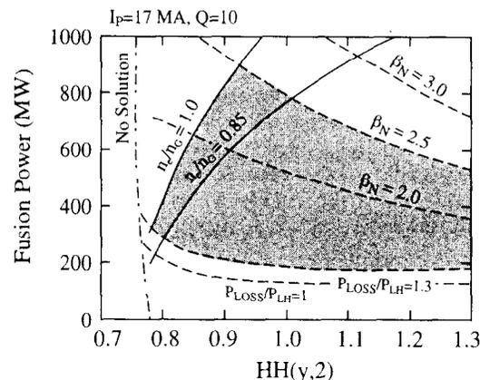
Fig. 14. The  $Q = 10$  operation domain (zero-dimensional modeling) with  $I_p = 17$  MA ( $\tau_{He}^*/\tau_E = 5$ , Be = 2%, Ar = 0.12%).
