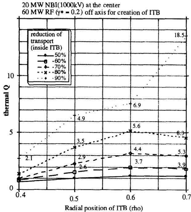
Fig. 11. Radial position of ITB and achievable thermal Q value.
