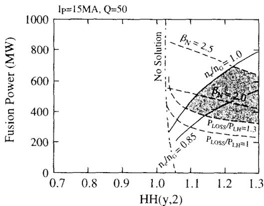
Fig. 15. The  $Q = 50$  operation domain (zero-dimensional modeling) with  $I_p = 15$  MA ( $\tau_{He}^*/\tau_E = 5$ , Be = 2%, Ar = 0.12%).
