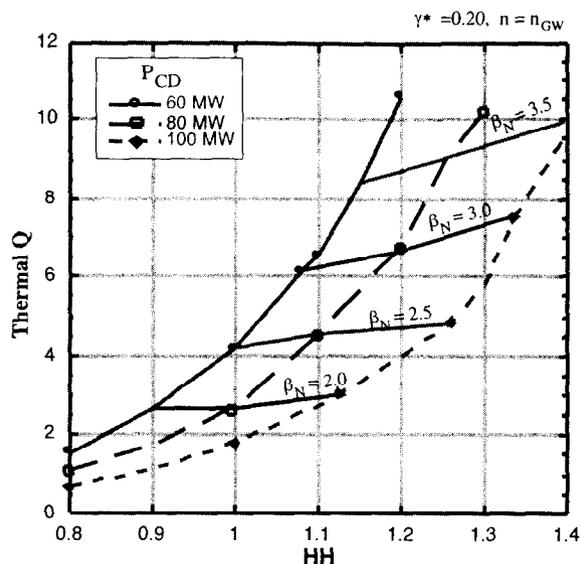
Fig. 9. Effect of CD power on the  $Q = 5$  operation domain.
