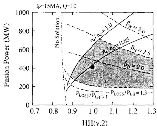
Fig. 13. The  $Q = 10$  operation domain (zero-dimensional modeling) with  $I_p = 15$  MA ( $\tau_{He}^*/\tau_E = 5$ , Be = 2%, Ar = 0.12%).
