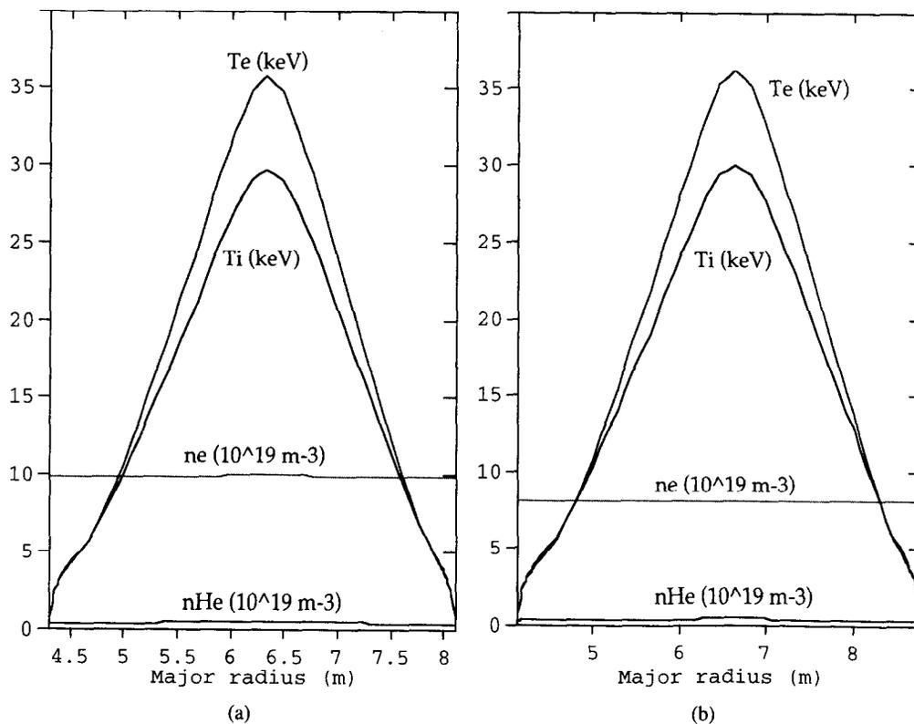
Fig. 4. Temperature and density profiles of (a) IAM and (b) LAM.
