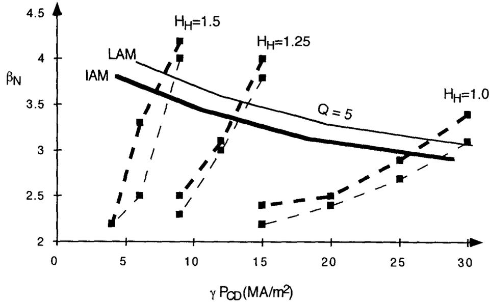
Fig. 12. Required  $\beta_N$  values as a function of CD FOM ( $\gamma \times P_{CD}$ ). The dotted lines indicate the constant  $H_H$  factor contours, and the solid lines indicate the constant  $Q = 5$  contours. IAM is indicated by thick lines, and LAM is indicated by thin lines. Two percent of carbon impurity is assumed.
