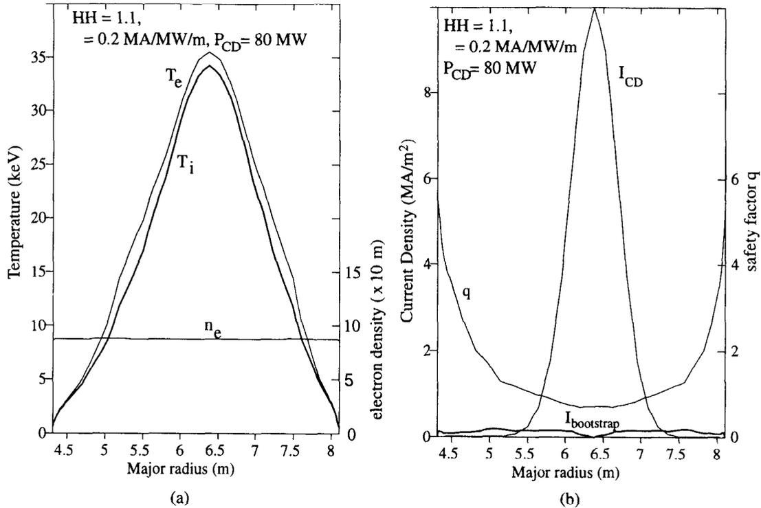
Fig. 7. (a) Temperature and density profiles and (b) current profiles and  $q$  profile of the noninductive operation simulated by 1.5-dimensional transport code.
