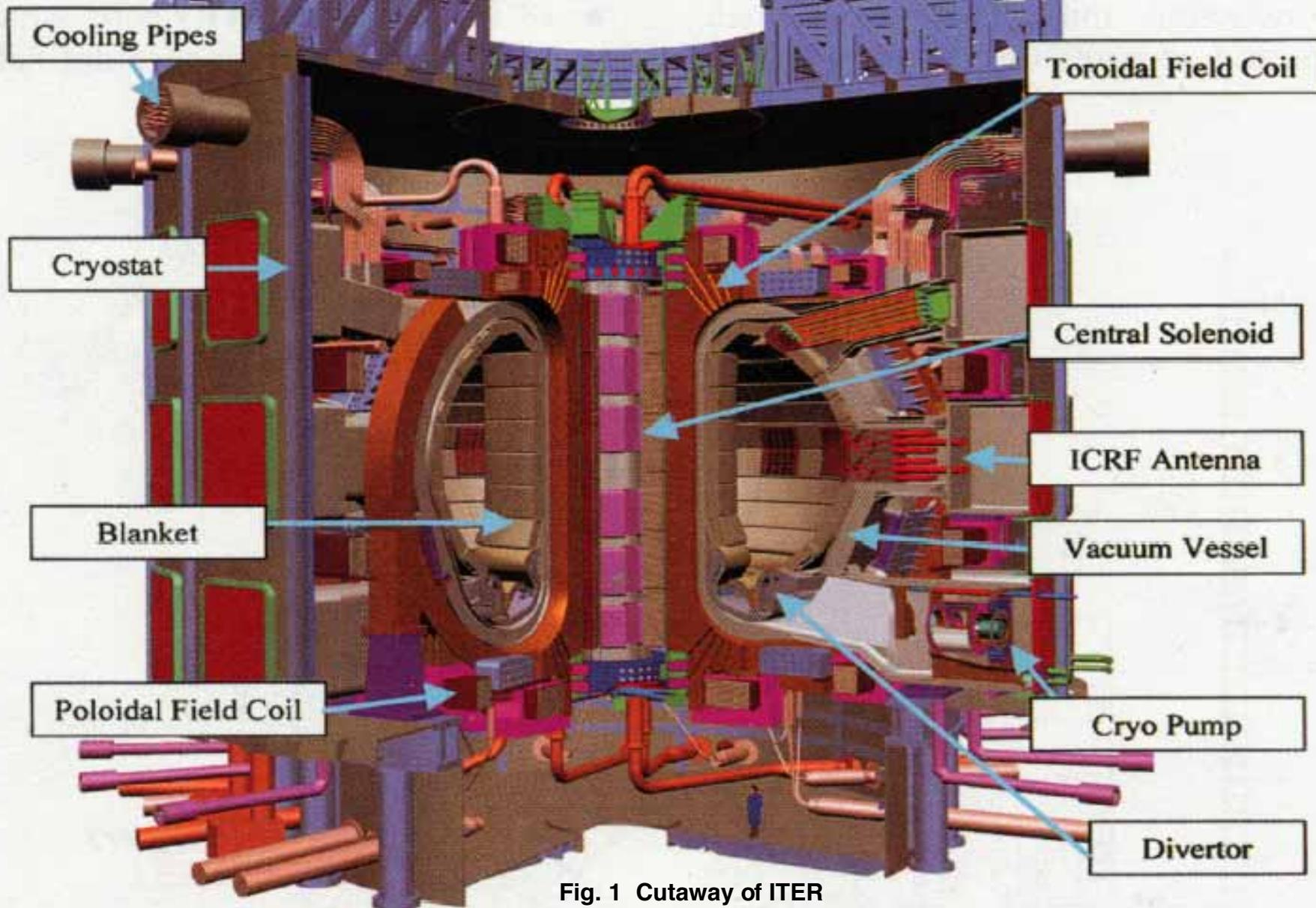
Fig. 1 Cutaway of ITER
