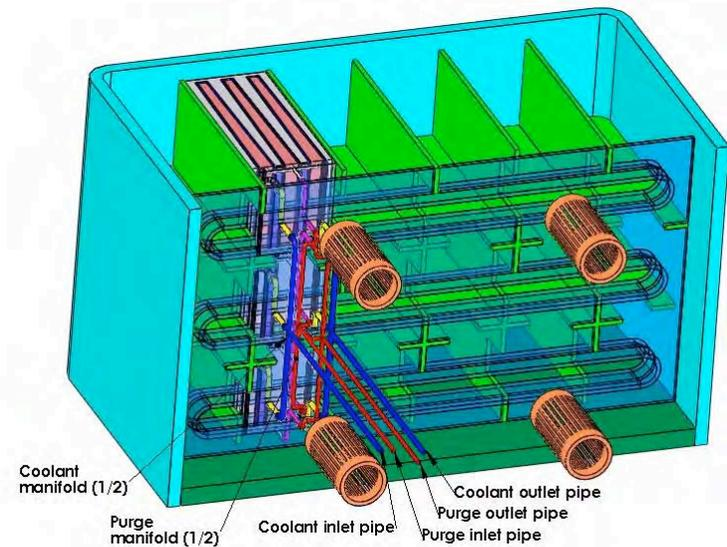
*Schematic view of three solid breeder thermomechanics unit cell test articles housed inside the EU's Helium-cooled pebble bed box*
