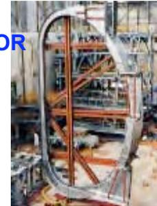
Double-Wall, Tolerance  $\pm 5$  mm
