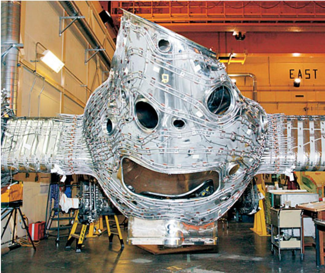
**The vacuum vessel** (segment shown) and other parts of the canceled stellarator at the Princeton Plasma Physics Laboratory have strange shapes to create quasi-symmetry for the plasma particles.
