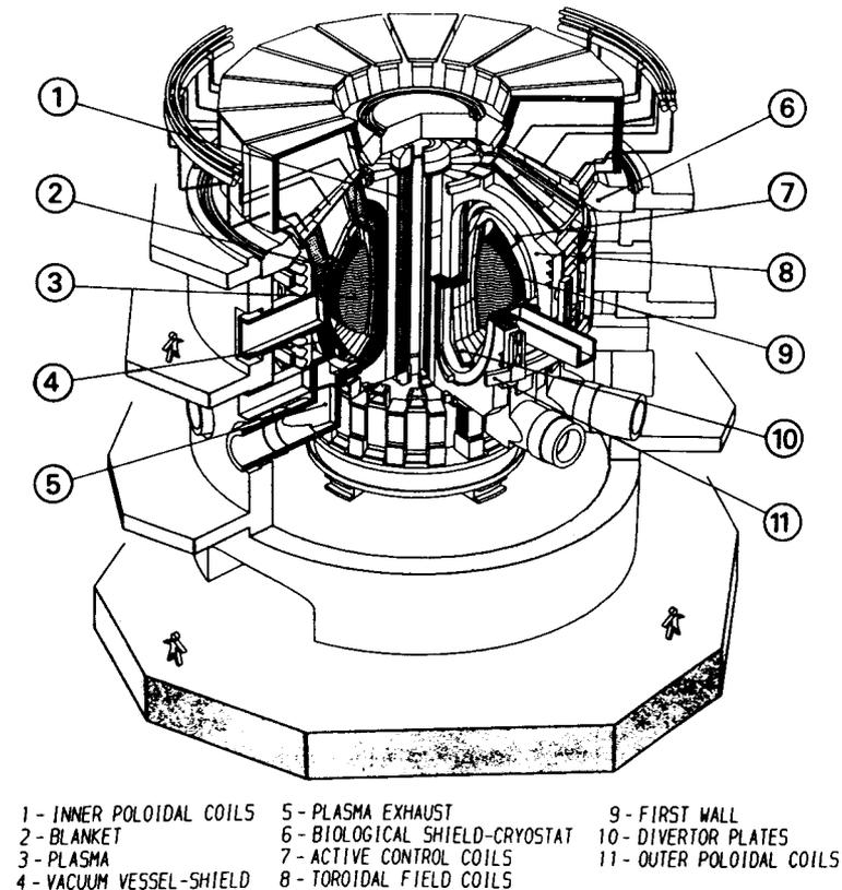
FIG. 1. An isometric view of NET device showing the main components.
