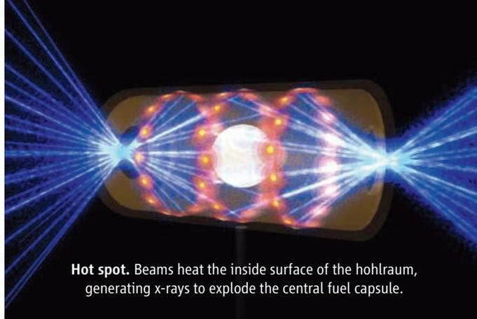
**Hot spot.** Beams heat the inside surface of the hohlraum, generating x-rays to explode the central fuel capsule.
