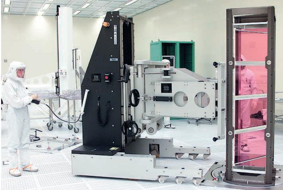
**Clean machines.** In conditions worthy of a semiconductor plant, technicians prepare a laser glass slab (right) for insertion into the beamline.
