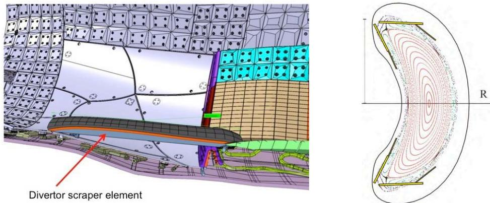
**Figure 3: Divertor scraper elements will protect the throat (narrowest part) of the divertor against heat transients during evolution of the plasma beta. The magnetic configuration near the island divertor plates, is shown on the right.**
