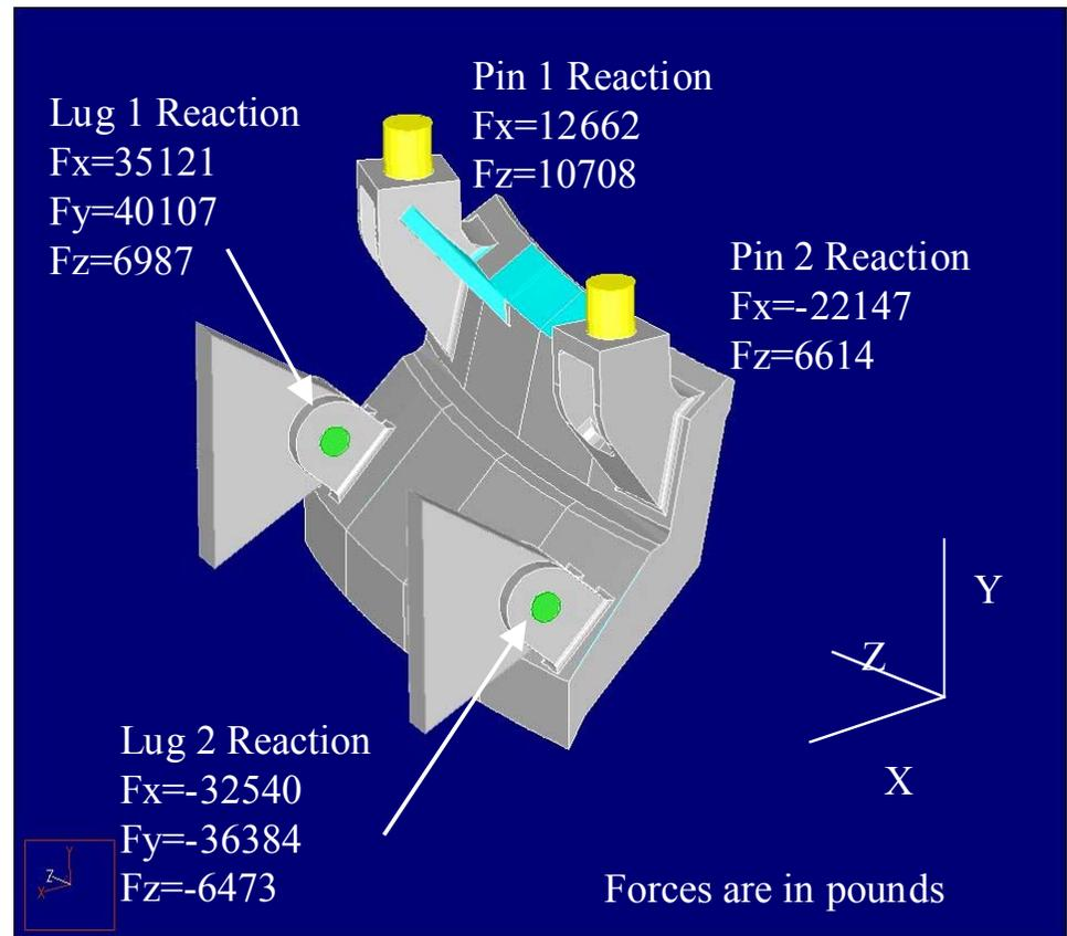
FIRE Vacuum Vessel and Remote Handling
