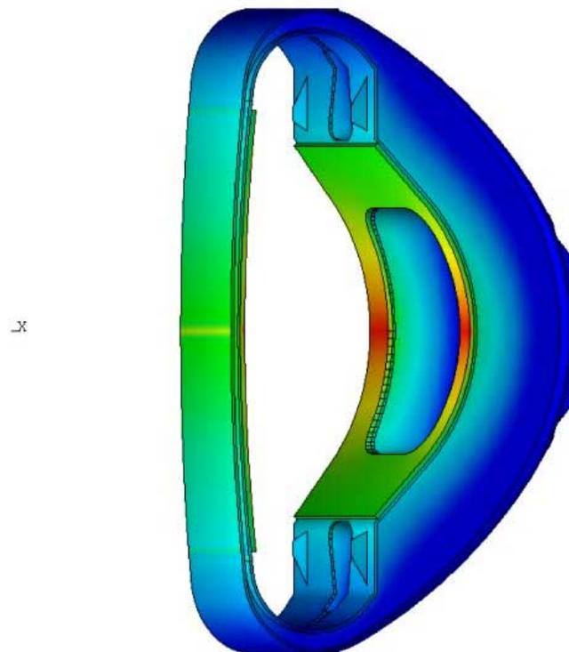
Thermal Load Due to Nuclear Heating
