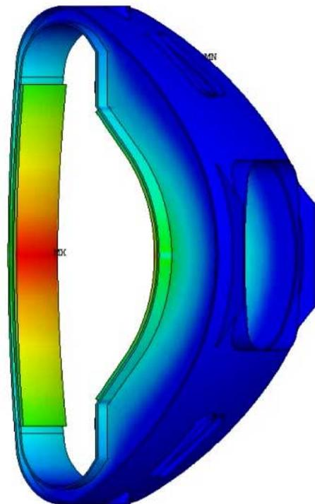
Thermal Load Due to Nuclear Heating
