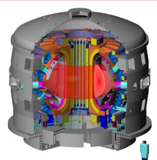
JT-60SC enclosed in a cryostat with a diameter of 12 m.
