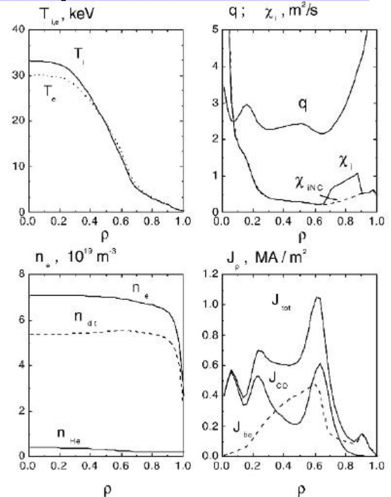
ITER's advanced scenarios are limited by conservatism rather than technical capabilities ( $P_{fus} \rightarrow 800 \text{ MW}$ ,  $P_{heat} \rightarrow 110 \text{ MW}$ )
