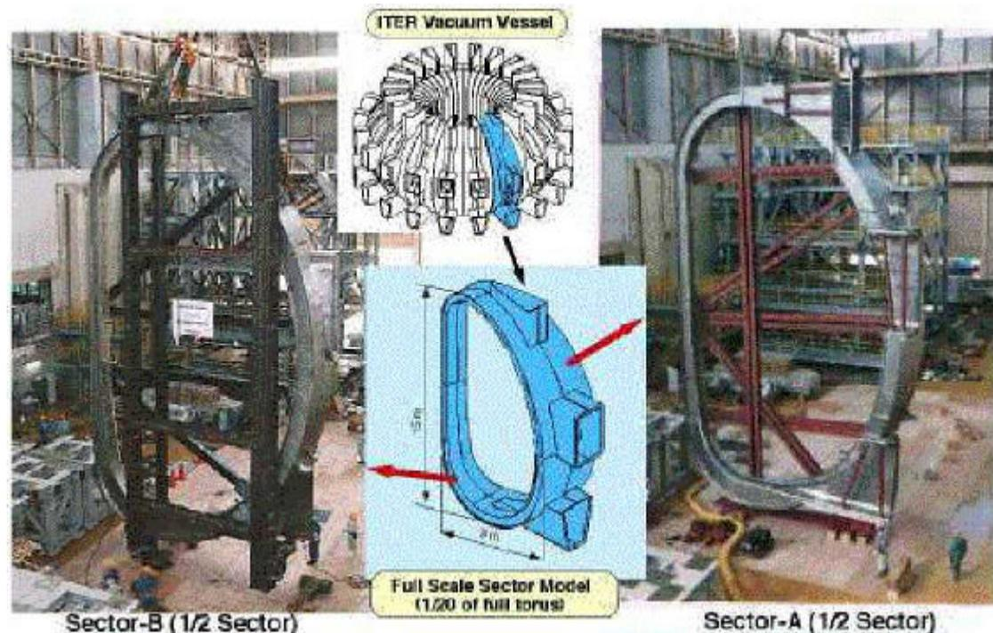
proof of accuracy in manufacturing and welding with 3 mm accuracy
