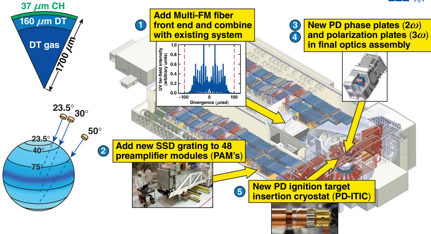
The laser technology required for polar-drive ignition on the NIF using a NIF PAM is being demonstrated on OMEGA EP.
