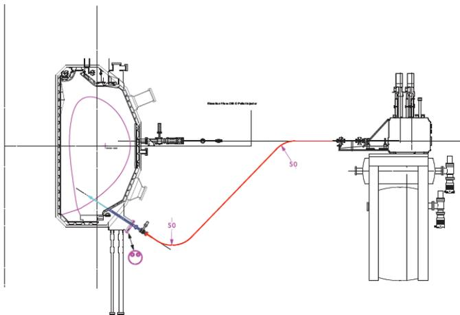
Pellet injection configuration on tokamak.
