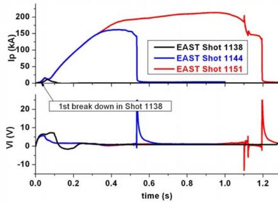
Fig.3 1<sup>st</sup> break down and following shots with  $I_p > 150$  kA and 220 kA
