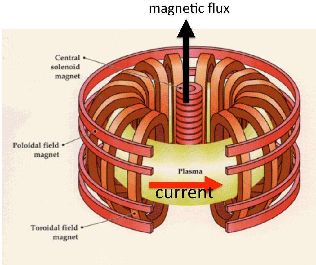
Magnets →  $B_{\text{toroidal}}$
