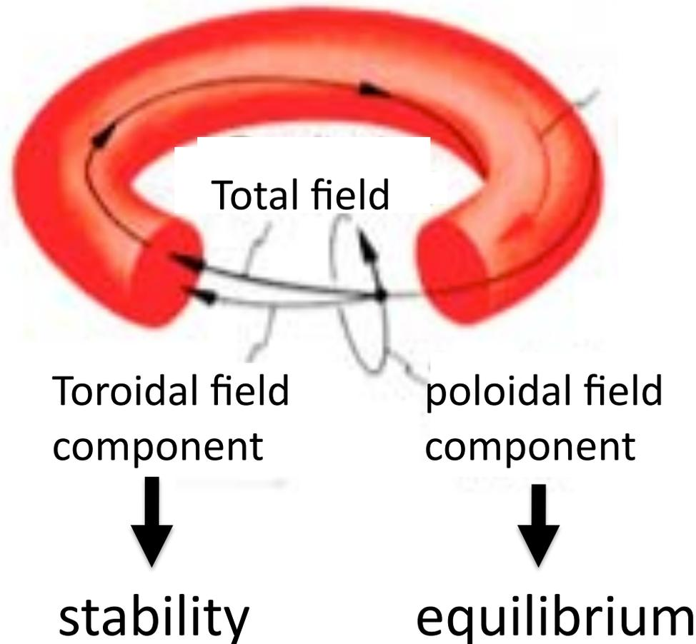
B is axisymmetric (2D), toroidal angle is ignorable,  $\frac{\partial B}{\partial \varphi} = 0$
