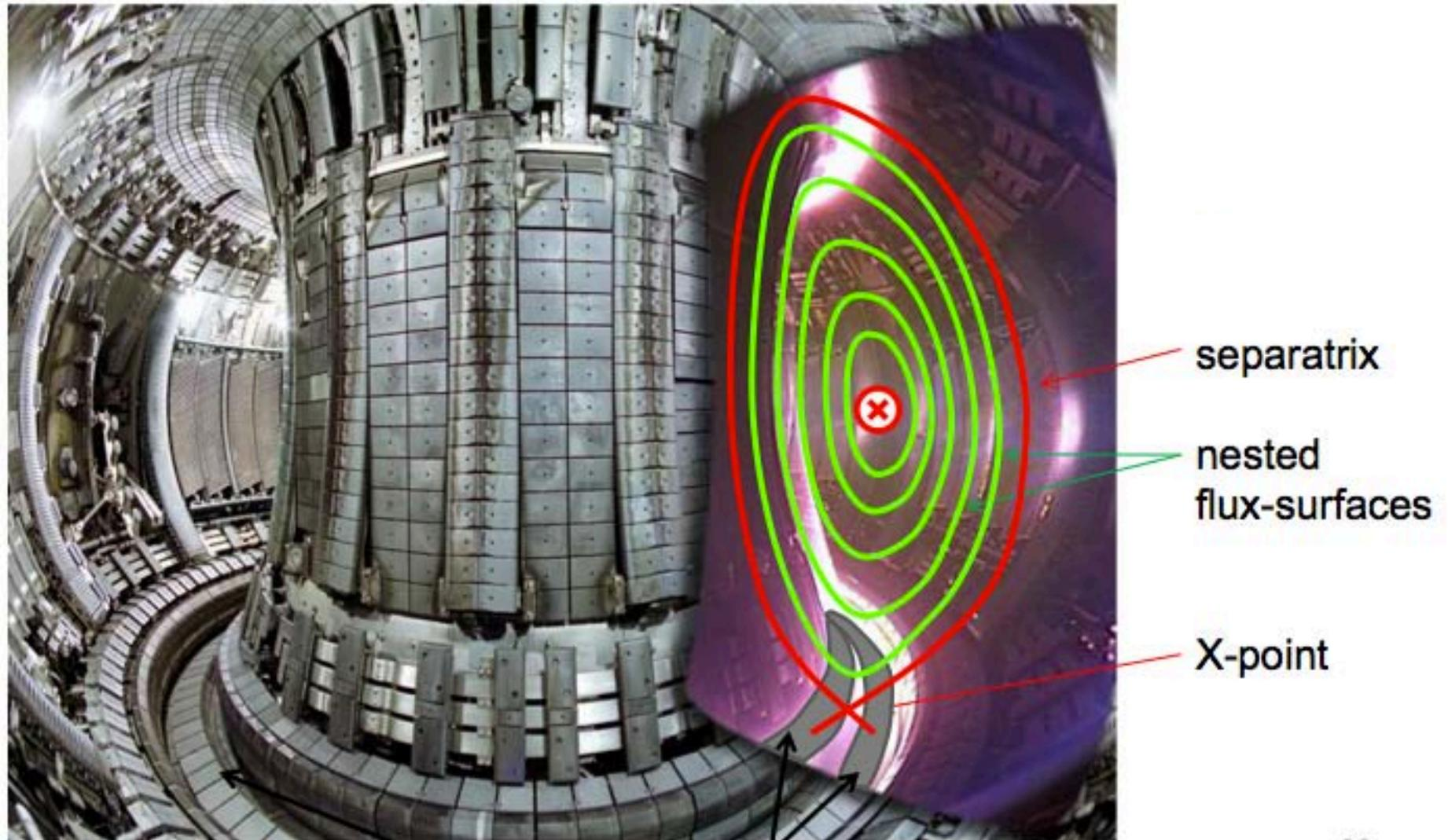
Divertor with target plates for exhaust
