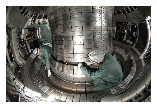
ASDEX Upgrade has pioneered modern tokamak operation with W-wall
