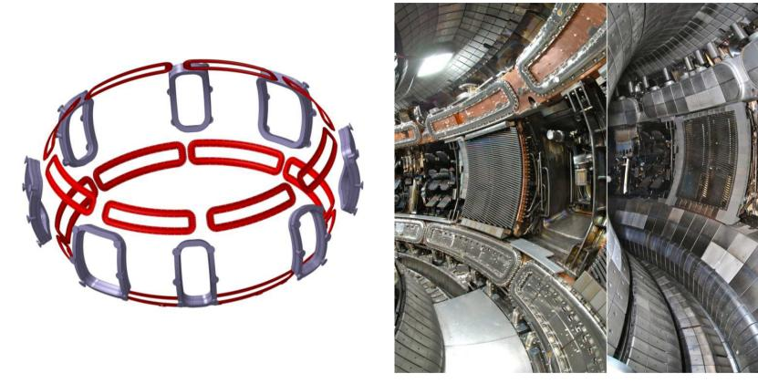
Flexible in-vessel coil system that allows n=1-4 perturbation fields
