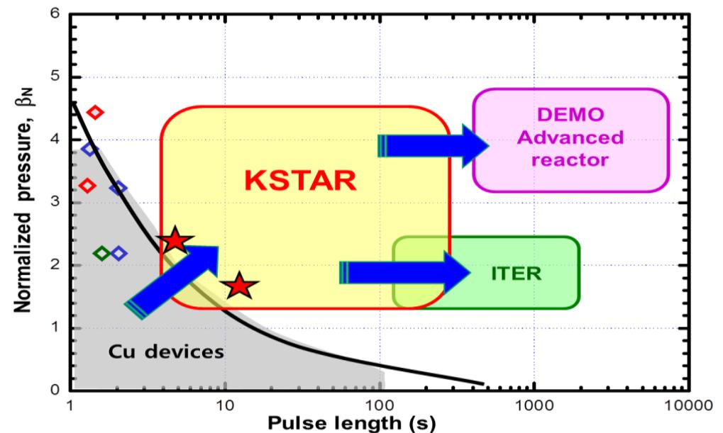
Machine design is optimized for **advanced** target operation
