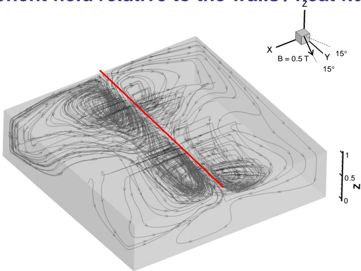
**Looking from the top, the heated spot appears to be pulled slightly off center line by strong lateral velocity**
