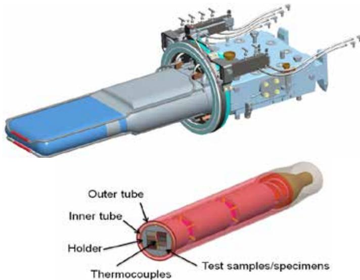
Active temperature control of material samples during irradiation
