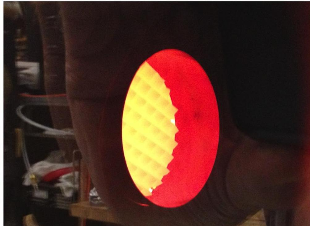
The Electron Cyclotron Emission (ECE) diagnostic contains a device used to calibrate the system. A Silicon Carbide disc is machined in a special way to have a pyramid pattern, shown on the left. This disc is then heated to well over 800°C. The right hand photo shows the calibration disc glowing red-hot while in use.
