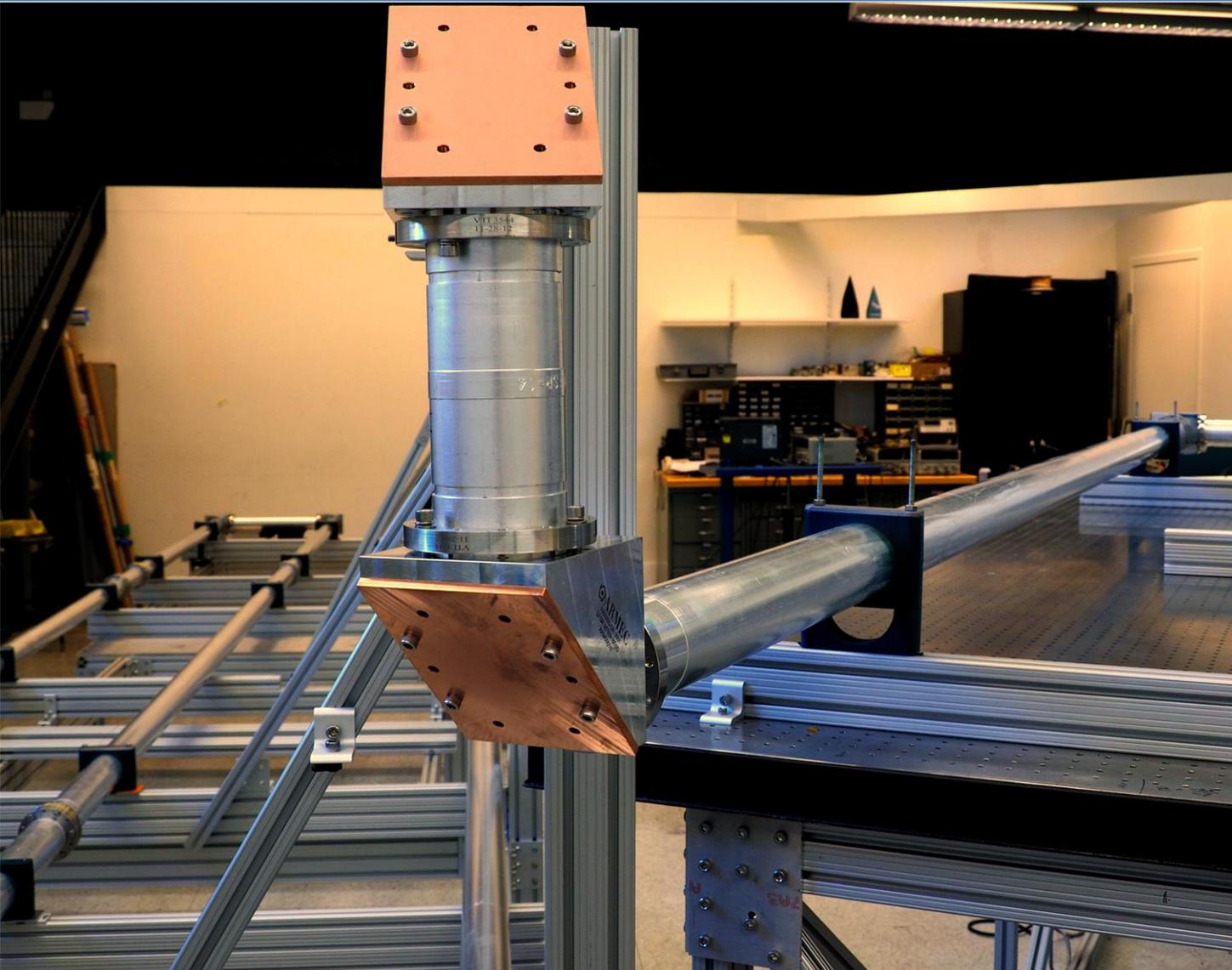
A test stand for the low-field-side reflectometer at UCLA mimics an ITER-like waveguide route; the copper material is part of a 30 degree miter bend. ORNL designed and fabricated the waveguide.
