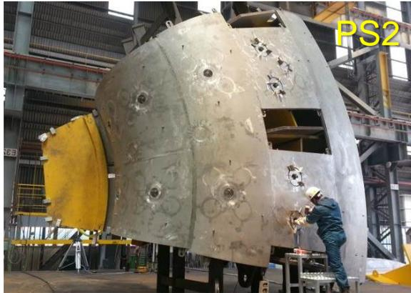
◀ Completion of welding of inter-modular and centering keys of inner shell of upper segment (PS2)
