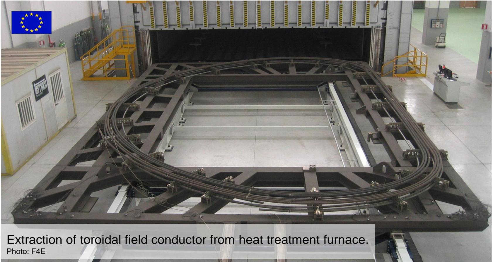
Extraction of toroidal field conductor from heat treatment furnace.
