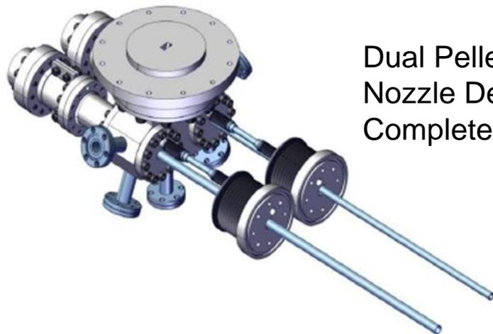
Dual Pellet Gun Nozzle Design Completed
