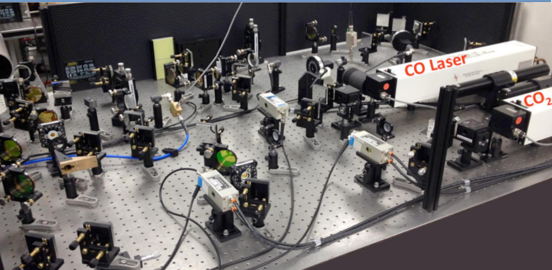
This complex optical table assembly is part of the Toroidal Interferometer and Polarimeter (TIP) diagnostic development at General Atomics in San Diego. The two lasers are injected in to ITER and the return signal is measured to determine the density of the plasma.
