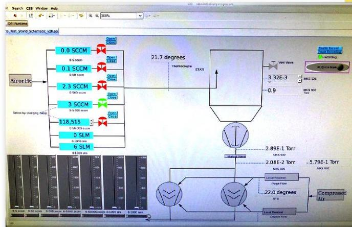
Data acquisition and control interface for roots and screw pump train
