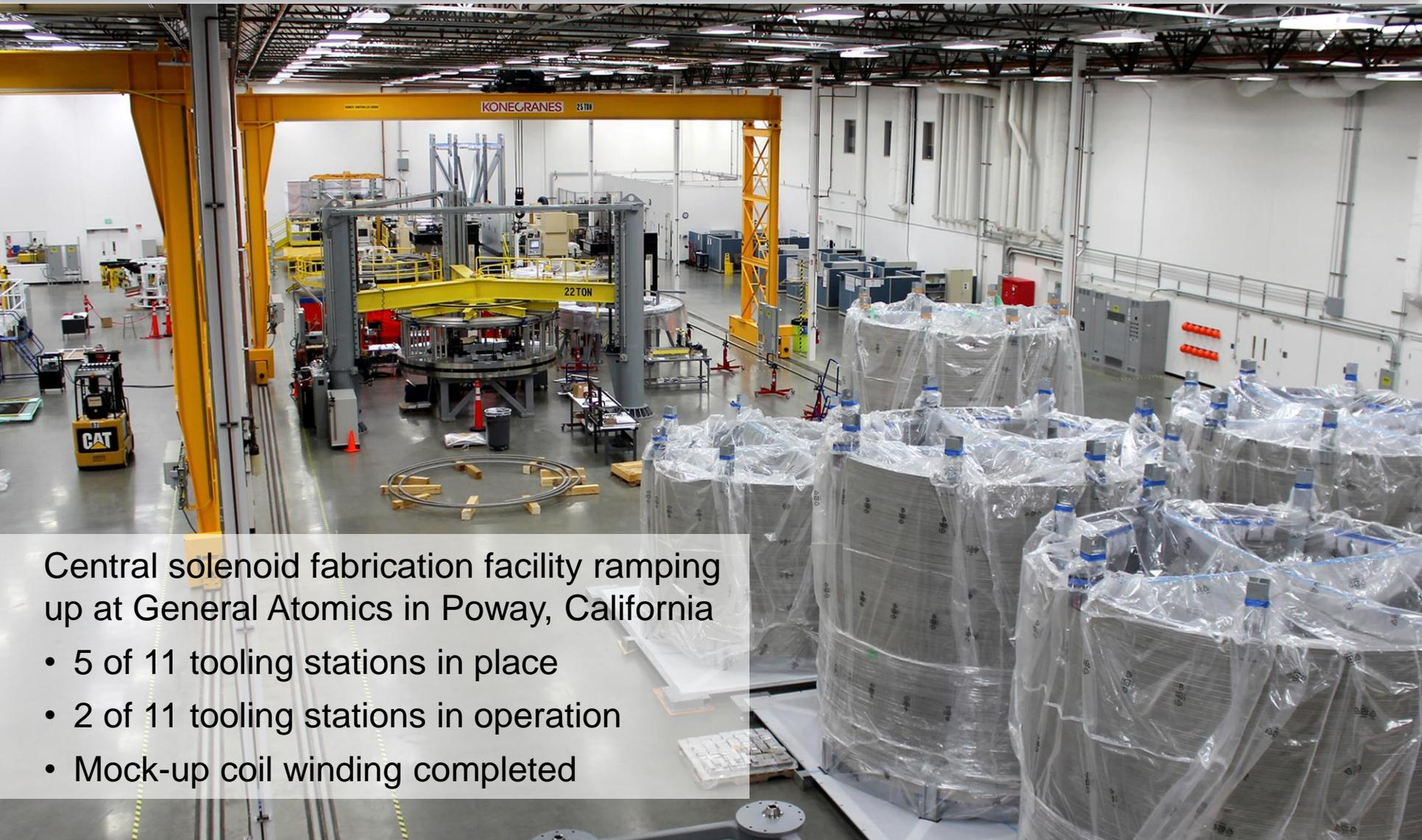
Central solenoid fabrication facility ramping up at General Atomics in Poway, California
