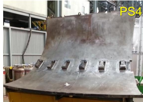
◀ Completion of forming of inner shell and machining of diverter rail, port stub corner, 4-pipe & IVV penetration of lower segment (PS4)
