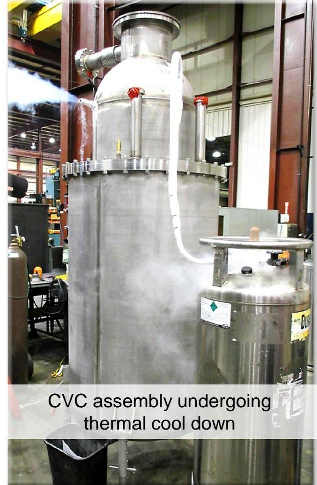
CVC assembly undergoing thermal cool down
