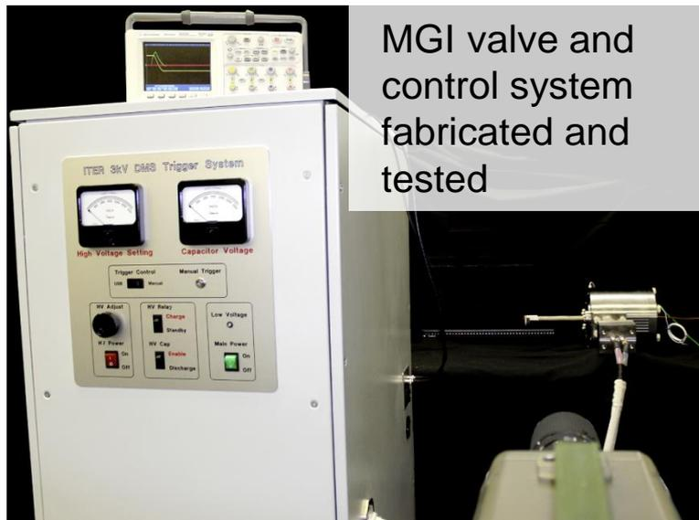
MGI valve and control system fabricated and tested
