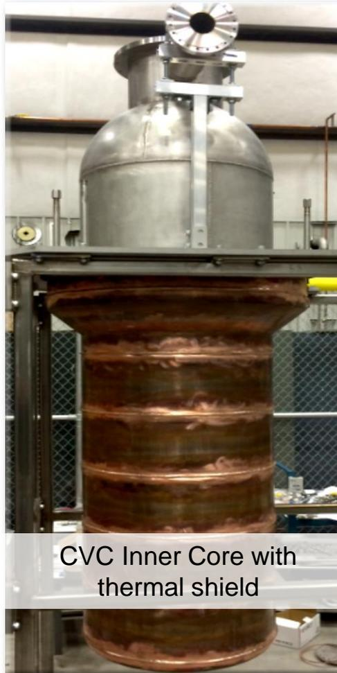
CVC Inner Core with thermal shield
