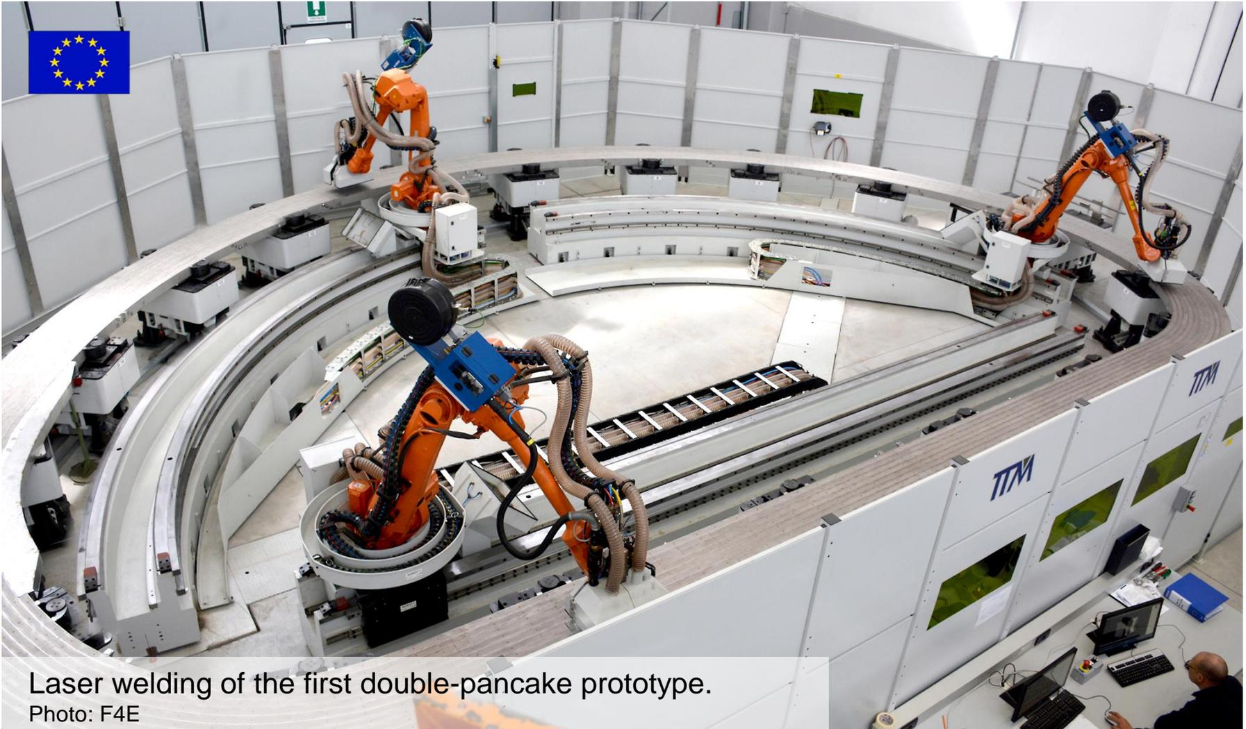
Laser welding of the first double-pancake prototype.
