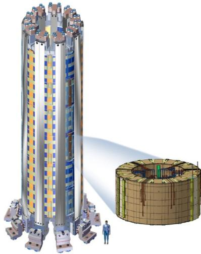
**1,000 metric ton magnet induces magnetic flux change needed to:**
