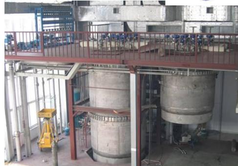
**2kW/4.5K Cryogenic & refrigerator system**
