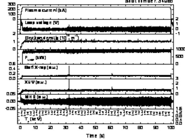
$I_p \sim 0.25$  MA, DN, elongation  $\sim 1.8$ , triangularity  $\sim 0.5$ ,
