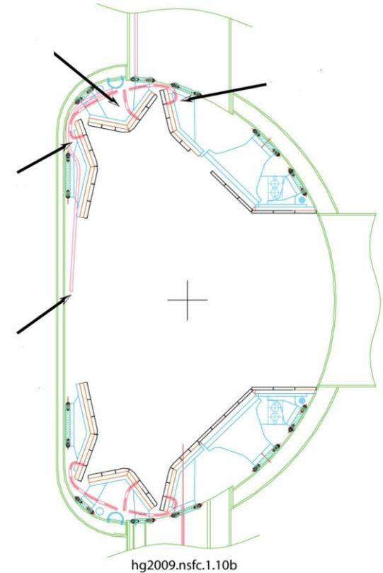
**DOME  $D_2$  puffing has highest fuelling efficiency, less from inner target plate, lowest from outer target plate. Compared to SN configuration, DN is more sensitive to gas puffing location.**
