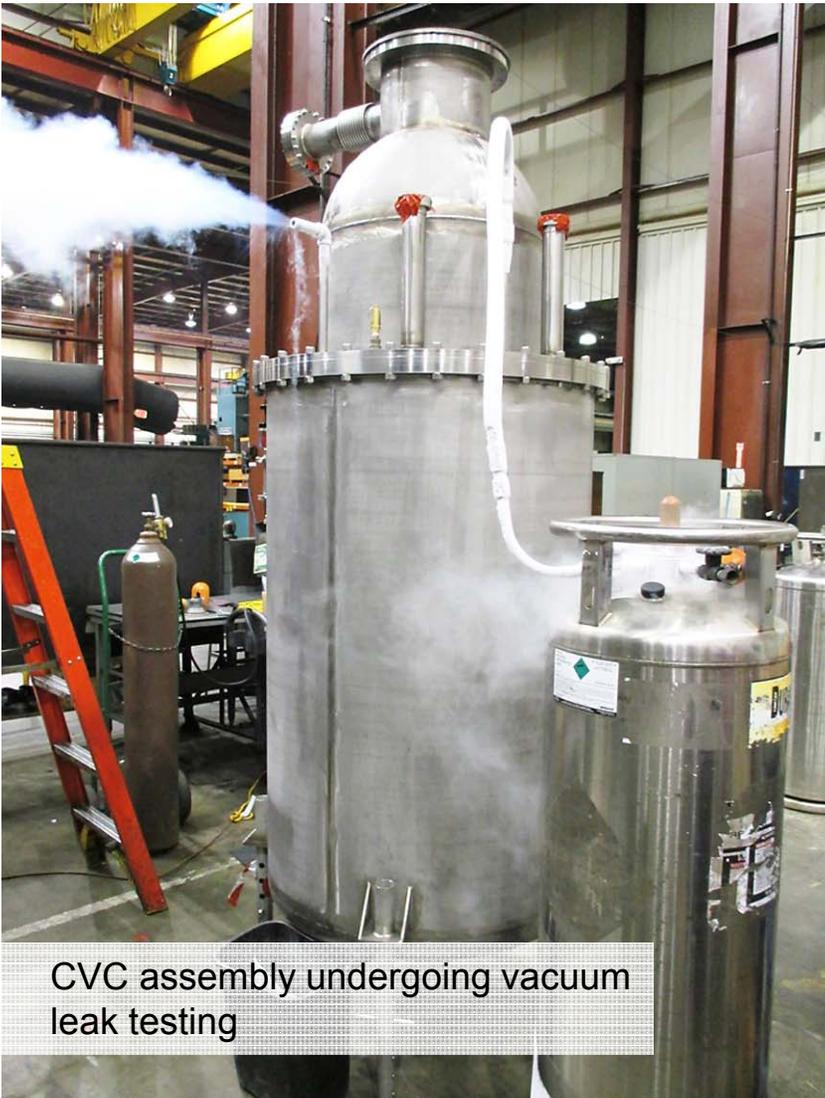
CVC assembly undergoing vacuum leak testing
