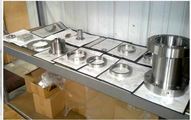
**Valve based on a design used on JET but modified for ITER tokamak environment and injection rate requirements.**
