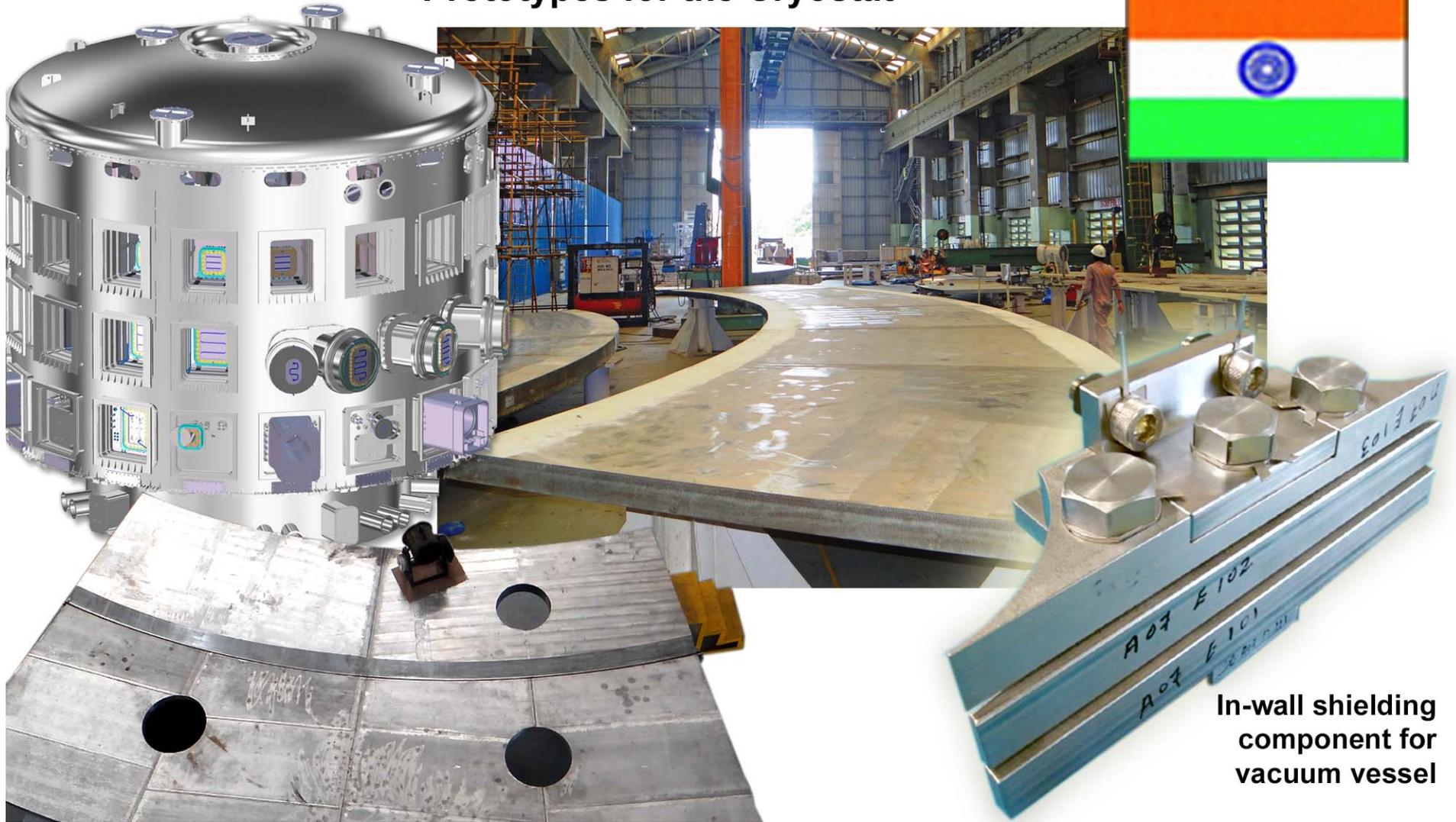
In-wall shielding component for vacuum vessel
