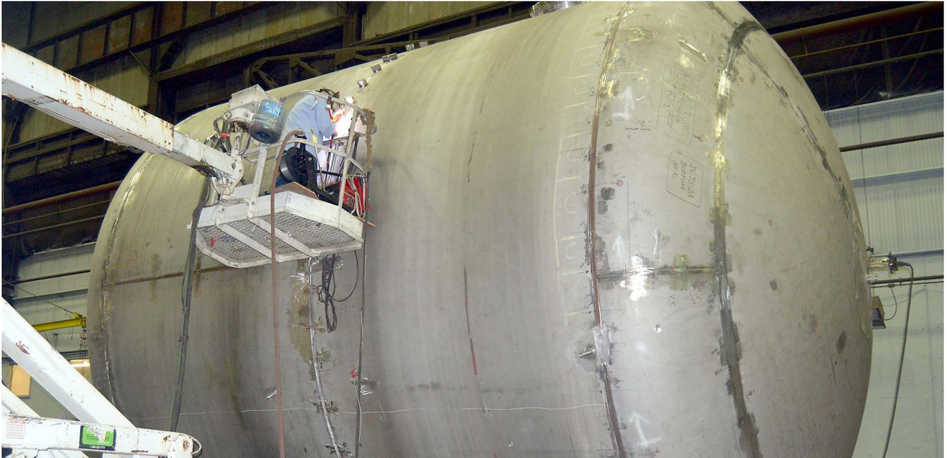
First of four 61,000 gallon drain tanks nears completion at Joseph Oat in Camden, New Jersey. (Fifth tank is ~30,000 gallons) Photo: US ITER
