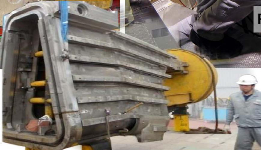
**Vacuum Vessel Port Fabrication**
