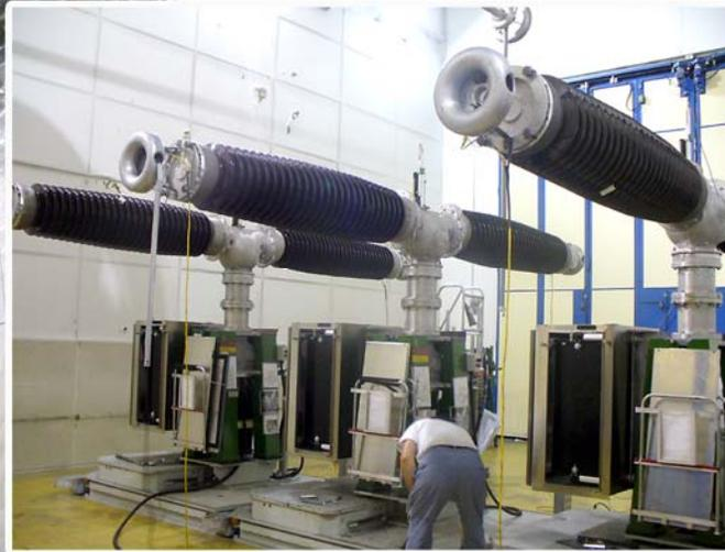
One of four sets of 400kV, 3-phase HV circuit breakers undergoing factory acceptance test at Alstom SAS, Villeurbane, France
