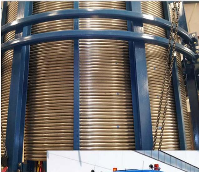
US TF 800 m Dummy Conductor and 100 m production conductor delivered to EU winding facility
