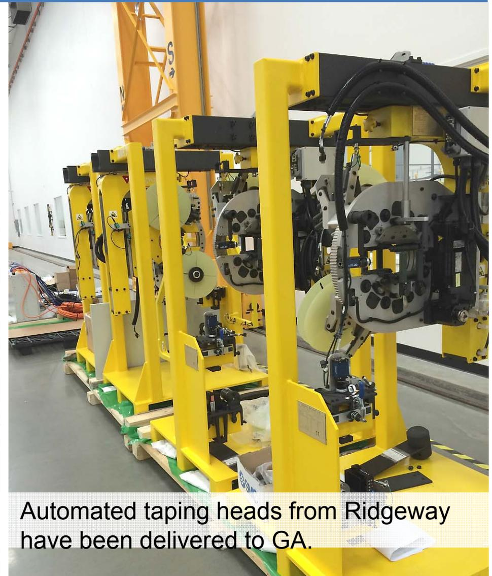
Automated taping heads from Ridgeway have been delivered to GA.
