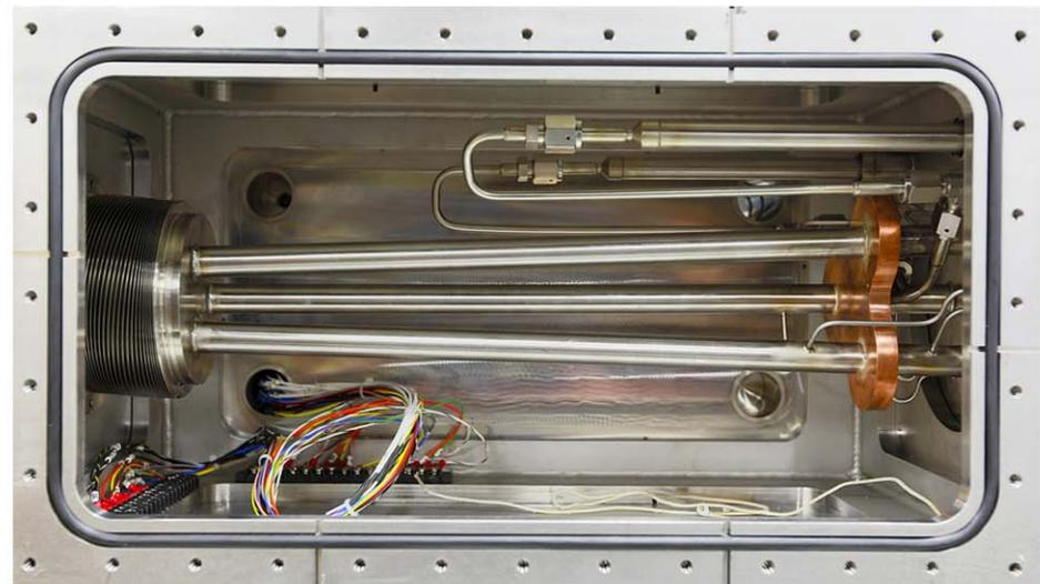
3-barrel unit prototype for disruption mitigation
