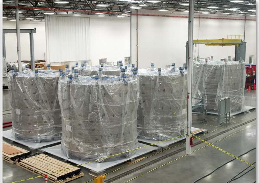
4 central solenoid active conductor spools and 1 dummy at General Atomics
