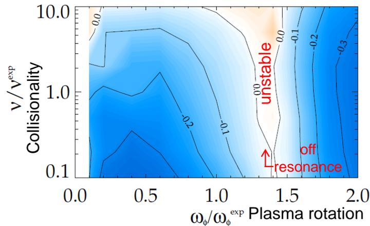
Figure 1: Computed effect of plasma collisionality on RWM stability (contours of normalized growth rate) as a function of plasma rotation, illustrating the effect of proximity to the ion-precession drift resonance.
