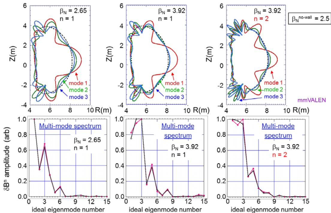
Figure 3: Multi-mode RWM analysis of ITER advanced scenario discharges, demonstrating a significant eigenmode spectrum in addition to the standard single ideal eigenmode typically assumed in control calculations.
