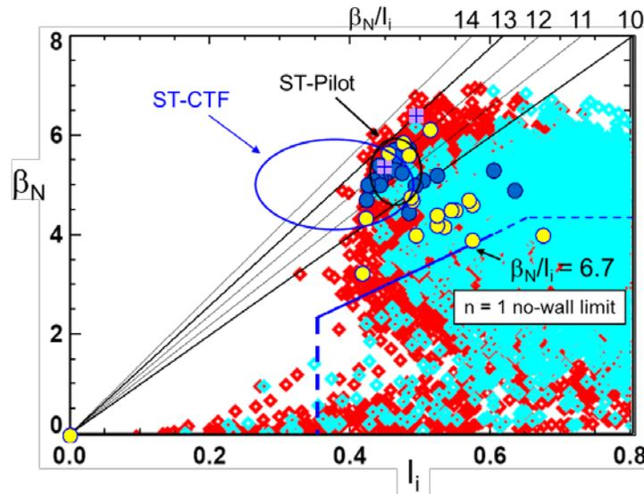
Figure 2: Operational stability space ( $I_i, \beta_N$ ) in NSTX illustrating a higher number of disruptions (yellow circles) at intermediate values of  $\beta_N$  in dedicated control experiments. The sharp reduction of the  $n = 1$  ideal no-wall stability limit as  $I_i$  is decreased is also shown, the vertical dashed line representing the approximate computed current-driven kink limit.
