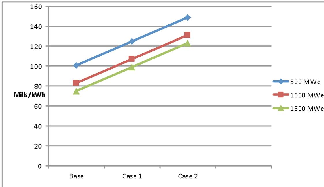
The base costs are for toroidal, cylindrical or spherical systems, excluding magnets and compression systems. Case 1, allows for an additional 1\$B in initial capital cost, i.e., before interest and owners costs. Case 2 is for 2 \$B. **Don't get hung up with the mills/kW.h. It's the relative values that matter.**
