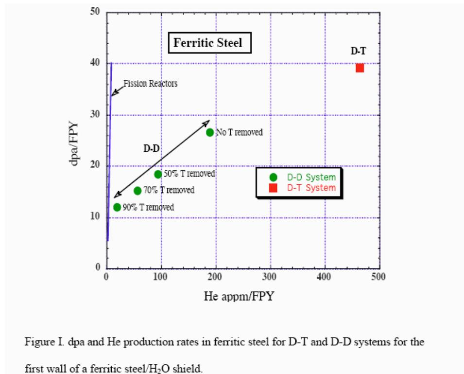
Figure I. dpa and He production rates in ferritic steel for D-T and D-D systems for the first wall of a ferritic steel/H<sub>2</sub>O shield.
