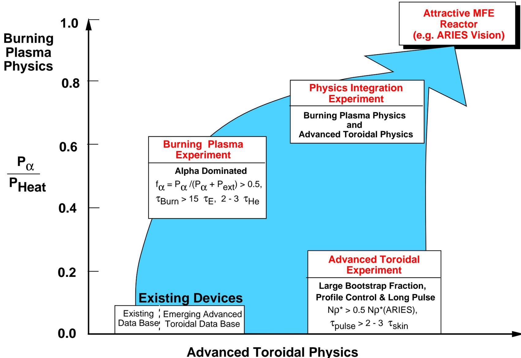
The “Old Paradigm” required three separate devices, the “New Paradigm” could utilize one facility operating in three modes or phases.
