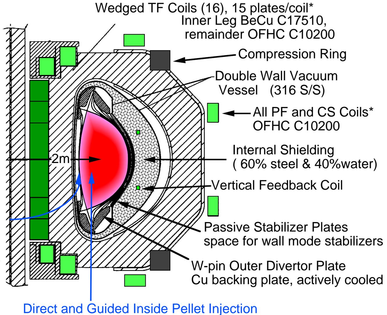
\*Coil systems cooled to 77 °K prior to pulse, rising to 373 °K by end of pulse.
