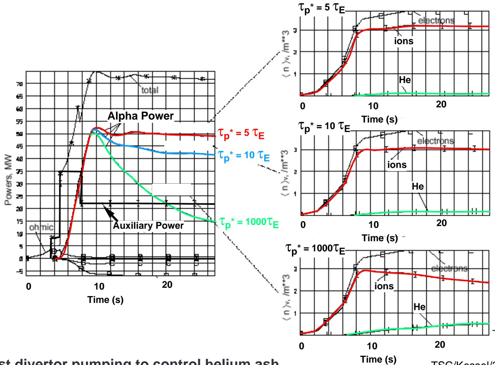
Adjust divertor pumping to control helium ash
