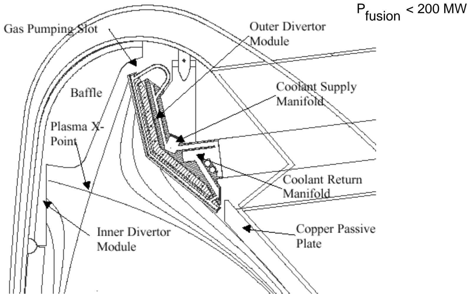
Reference Design is semi-detached operation with <15 MW / m<sup>2</sup>.
