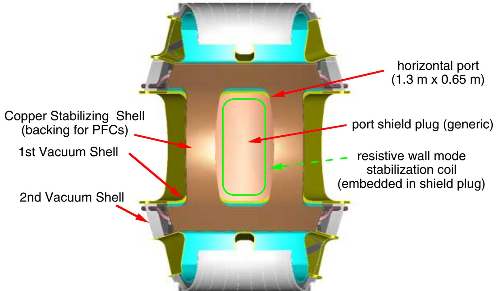
Concept under development by Columbia Univ. J. Bialek, G. Navratil, C.Kessel(PPPL) et al
