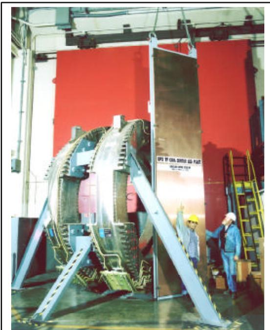
**Fig. 8.0-1. C17510 Copper Plate Produced for BPX.** Its size and properties are similar to that required by FIRE.
