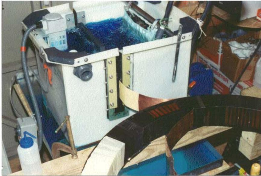
Figure 5.2-7 Electroforming the terminal flag onto one of C-Mod's strip wound poloidal field coils. The process of forming the inner joint of FIRE's CS double pancake assembly would be very similar, with the spiral cut pancakes expanded to allow access for a plating tank. Rubber sealed slots to allow the inner turn to be inserted in the tank. (Ed. Fitzgerald C-Mod Photo)
