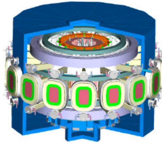
(a) Cross-Sectional View of FIRE Through Its Insulation Enclosure
