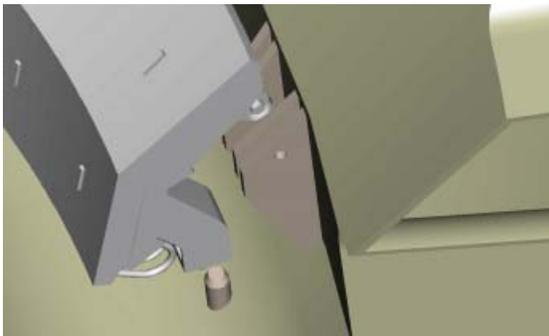
Figure 5.4.3.2.3-2 Divertor Module In-Position to Engage Vessel Attachment Hardware.
