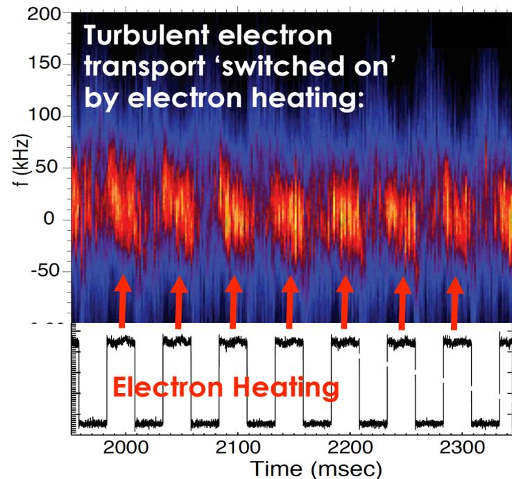
**Microwave upgrade (~ 8 MW to 15 MW) will access burning plasma relevant transport regimes**
