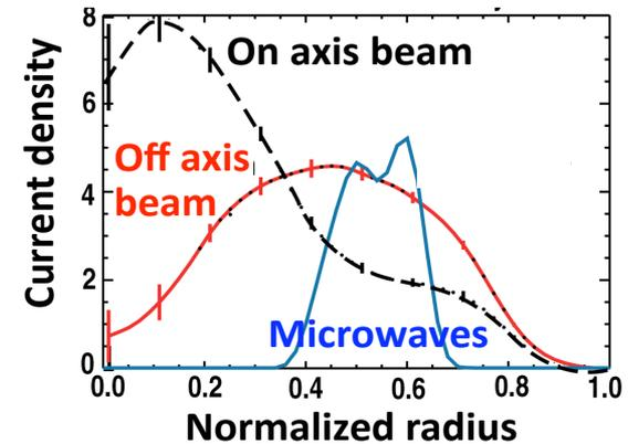
**Off-axis neutral beams & microwave driven currents provide off-axis current**
