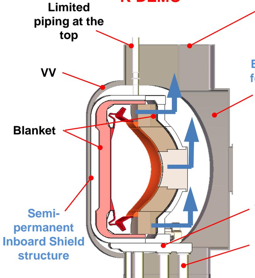
In-vessel component maintenance access
