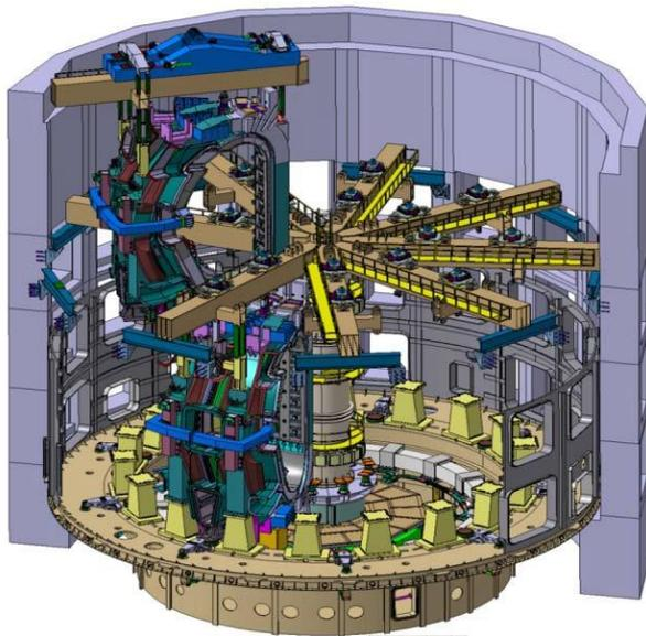
Assembly within the tokamak pit
