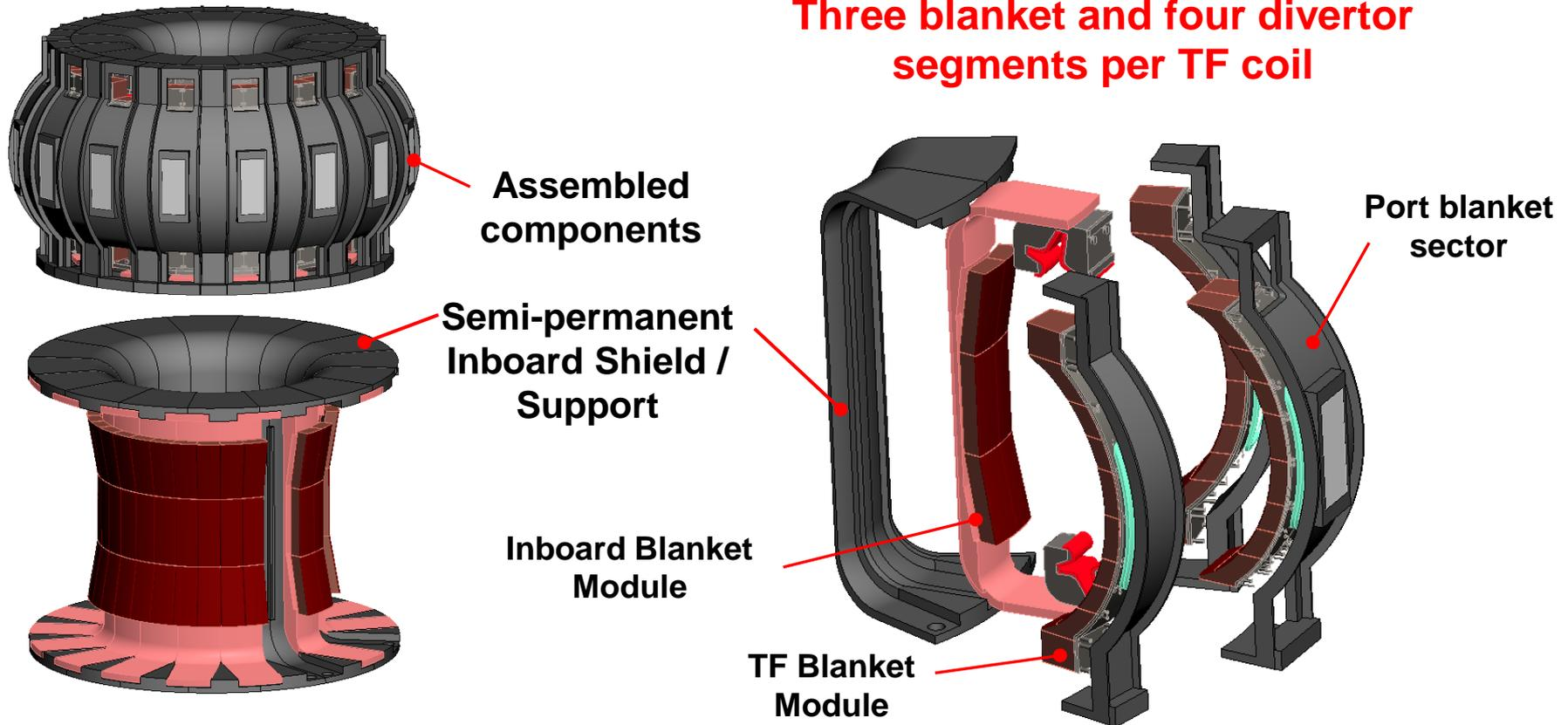
**Semi-permanent inboard shield used for alignment, disruption load support and shielding for gaps between modules**
