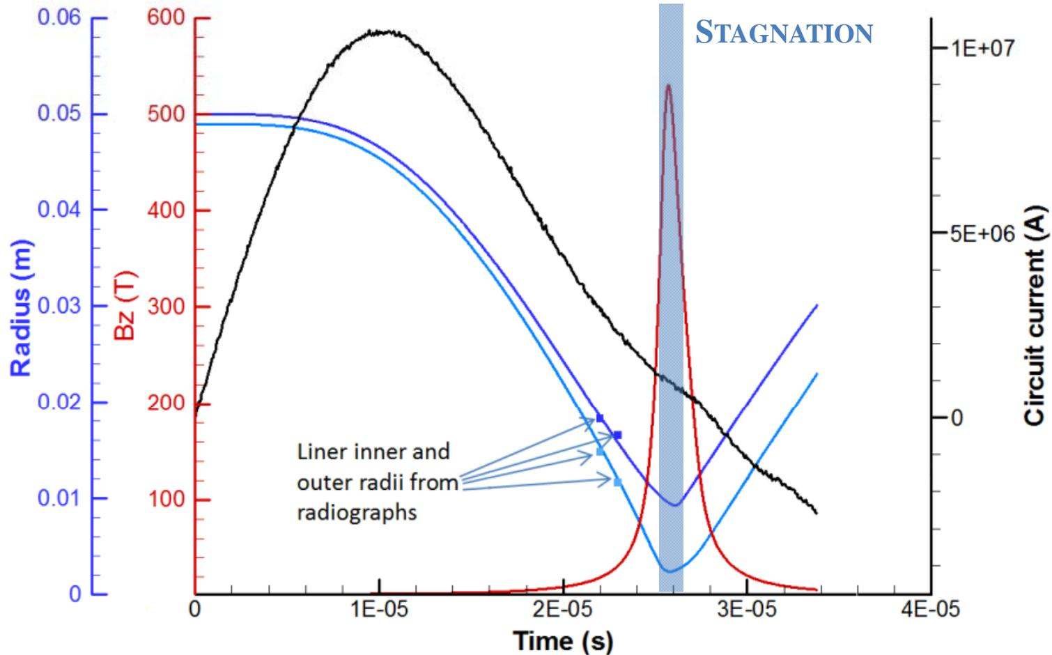
Note: The “bump” in the current trace (black) was predicted by modeling, and is observed in the experiments. It is caused by the rebound of the liner off of the magnetic field.
