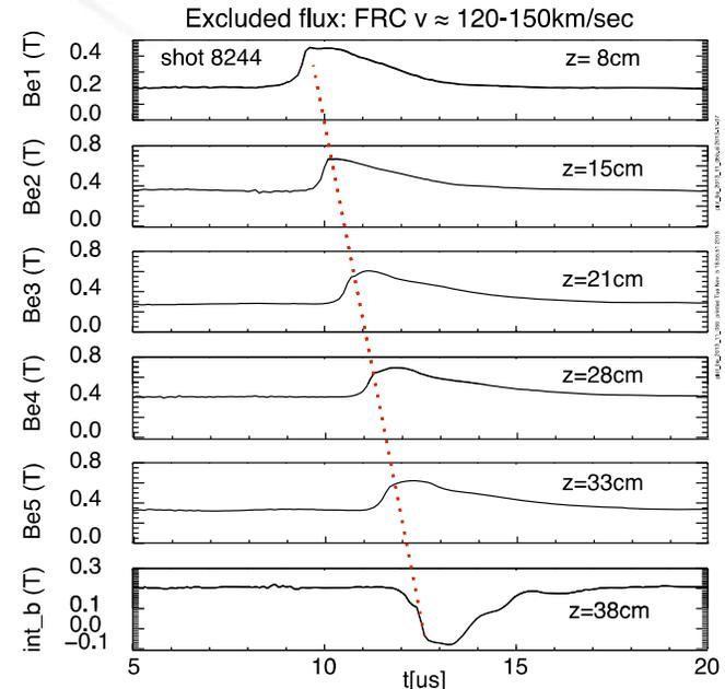
*external B probe array data shows FRC speed*
