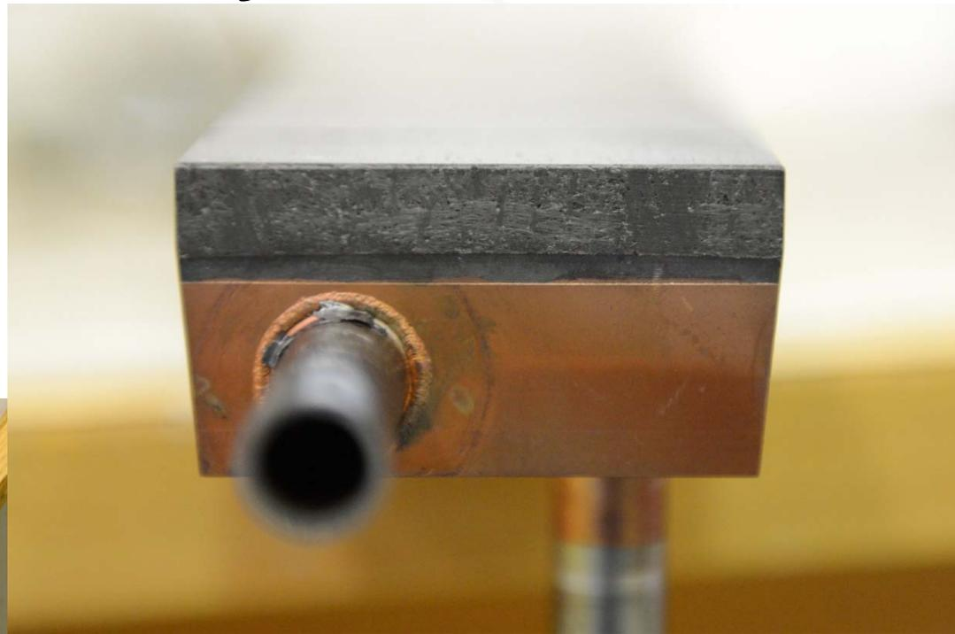
Above: The CuCrZr bonding layer is visible between the CFC graphite and copper substrate.
