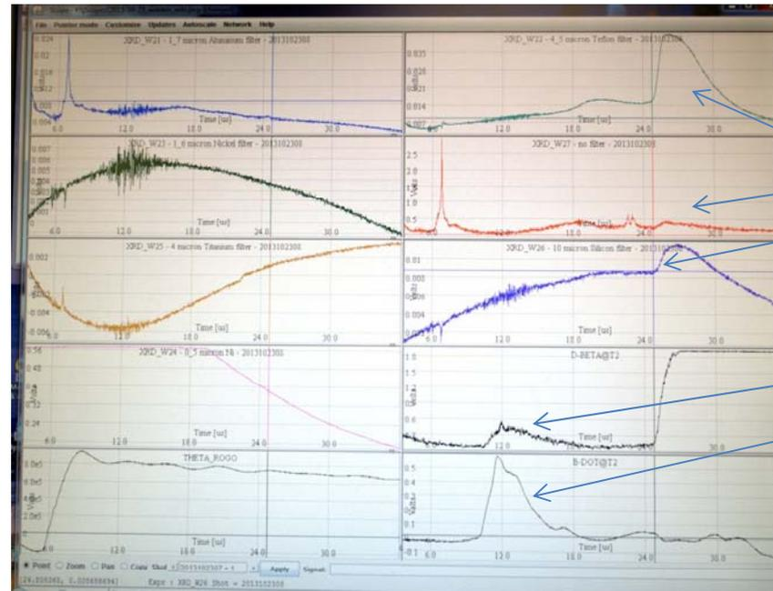
Filtered XRD photodiodes take off at 24.8 usec
