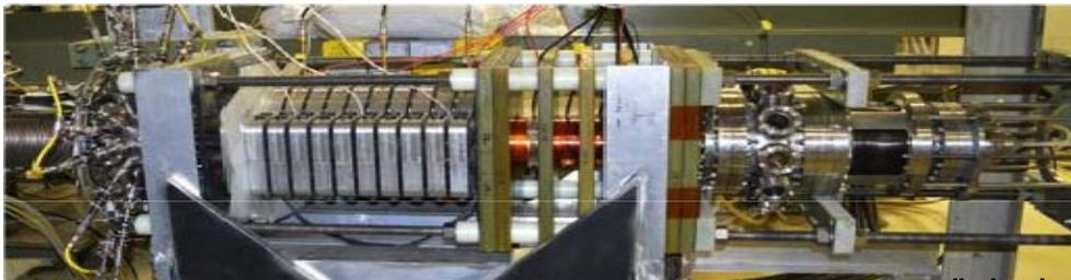
$\theta$  pinch formation      FRC acceleration: with segmented  $\theta$  coils      FRC drifts through vacuum      **perpendicular shock:** FRC stagnates onto compressed mirror field
