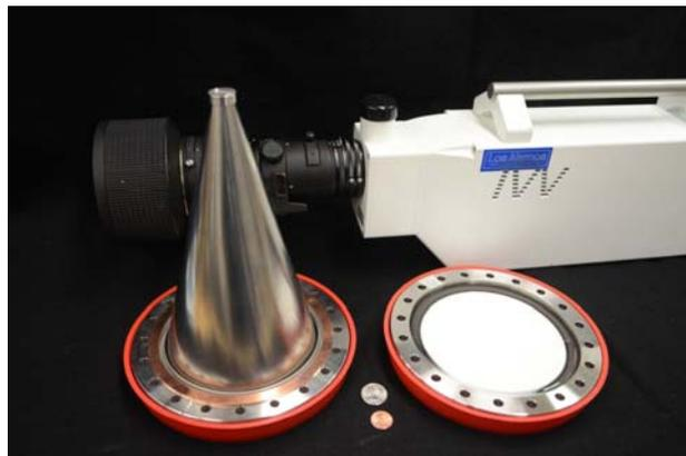
A P46 phosphor converts VUV and soft x-ray light into visible light, imaged by a telephoto lens on the Hadland camera (2 usec exposure for each frame)
