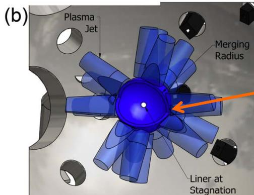
Imploding spherical plasma liner formed by 30 merging jets
