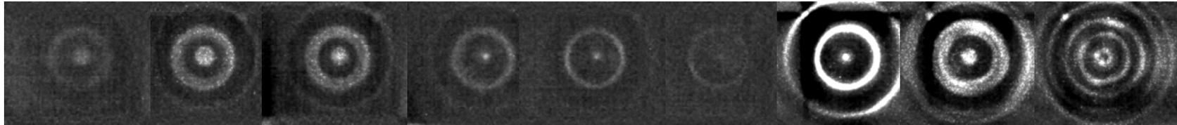
The FRC plasma is the central feature, the middle ring is a reflection from half-way down the column. It certainly compresses, but also fades until the 7<sup>th</sup> frame (stagnation time). Expansion (rebound) is seen in the last two frames shown here.
