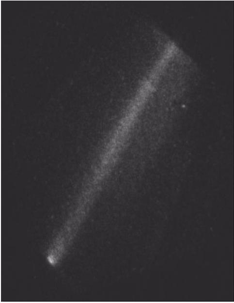
Z=25cm from plasma gun  $J_z(x,y)$  flux rope (black) & reversed (white)
