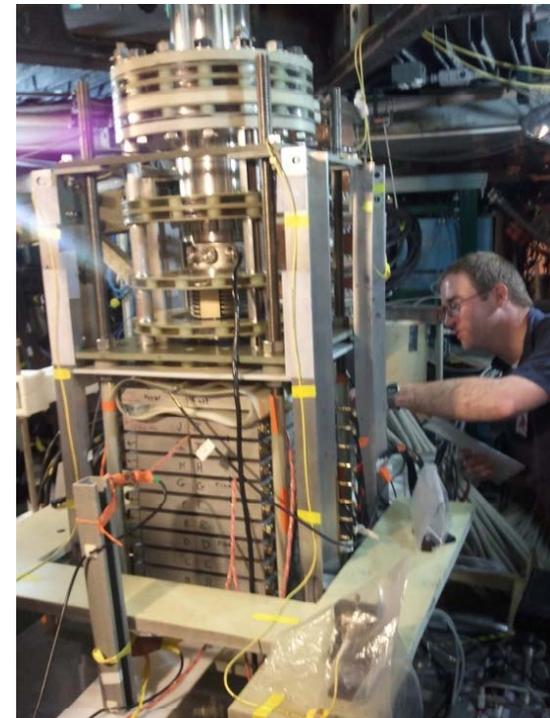
Shiva Star (left) can store 9 MJ of energy with 1.3 mF of capacitors, at up to 120kV. More typically, at 4.5 MJ, it delivers 11.4 MA of current to crush a 30-cm tall, 10 cm diameter, 1 mm thick, 270 gm Aluminum cylindrical liner load in 25 microseconds. The FRCHX load assembly (right) is located under the center of Shiva Star.
