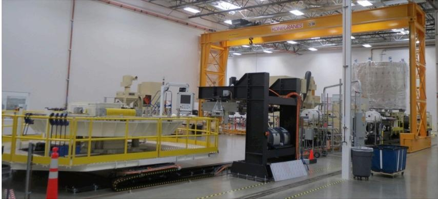
Two parallel lines can wind the 49mm square jacketed superconductor into 14 turn pancakes
