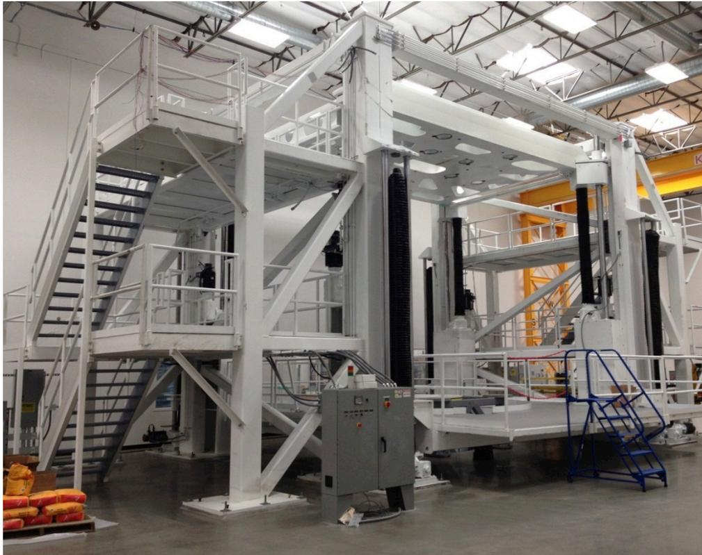
Automated wrapping system for applying insulating tapes →
