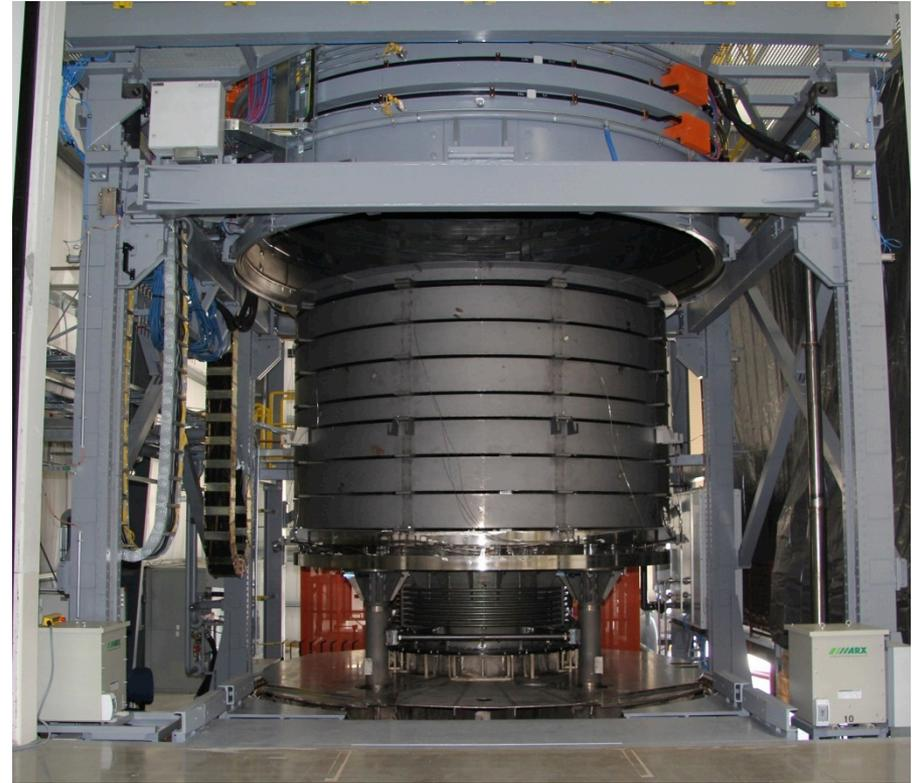
Argon atmosphere furnace for heat treating superconductor. A geometric representation of CS Module is used to qualify the convection furnace for operation with the coils
