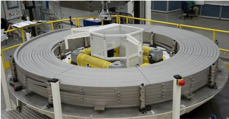
Prototype coil winding: 900m of continuous winding forms 6 out of 40 coil layers
