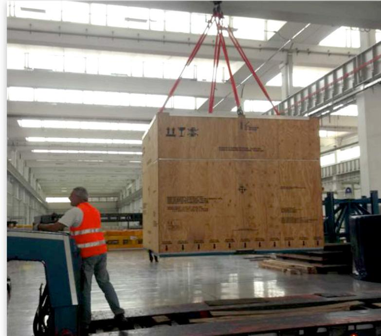
US TF 800 m dummy conductor – delivery at ASG in Italy
