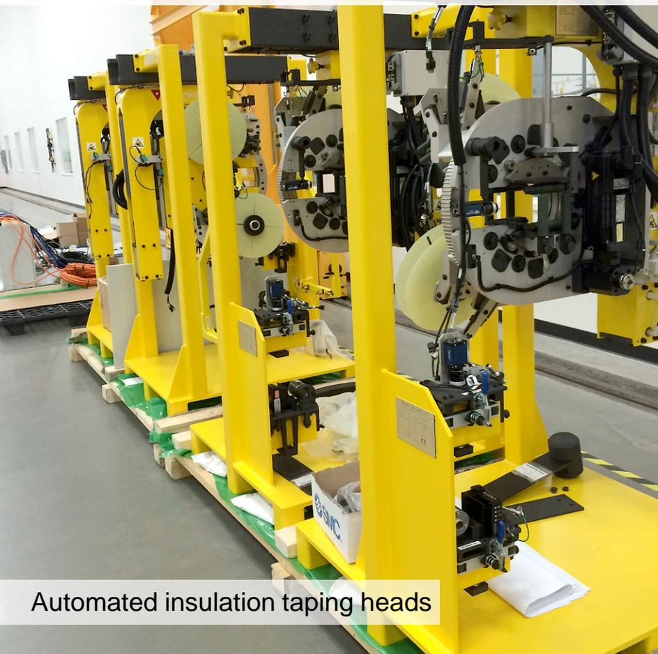
Automated insulation taping heads
