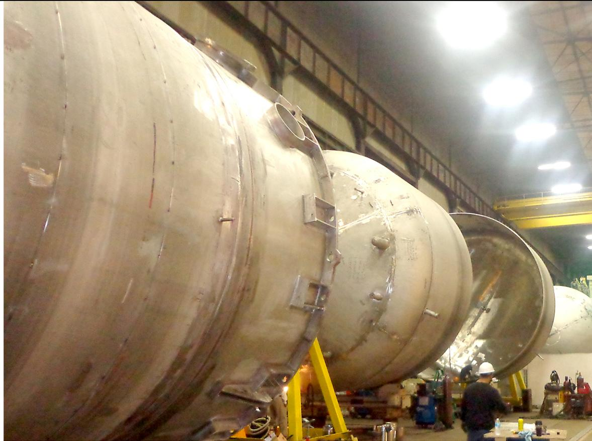
All drain tanks (four 61,000 gallon drain tanks and one ~30,000 gallon tank) will complete fabrication by February 2015. At left, a completed tank undergoes a lifting test. At right, tanks in earlier stages of fabrication.
