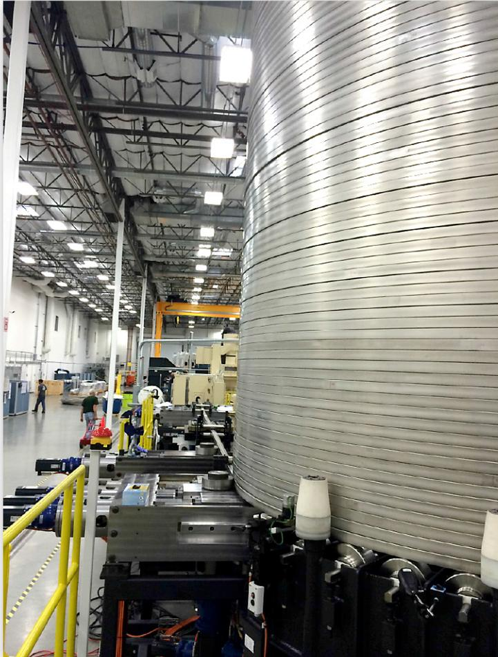
Conductor routed from the de-spooler of the winding station
