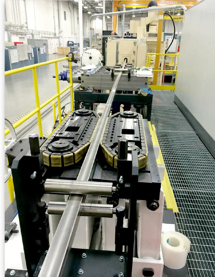
Conductor routed through tractor drive to the straightener
