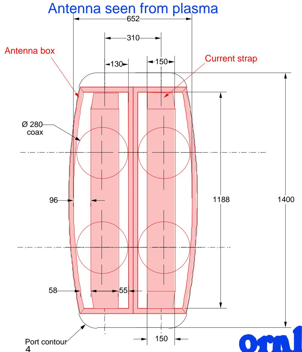
Each antenna contains shielding to reduce radiation at outside flange so that hands-on maintenance can be done
