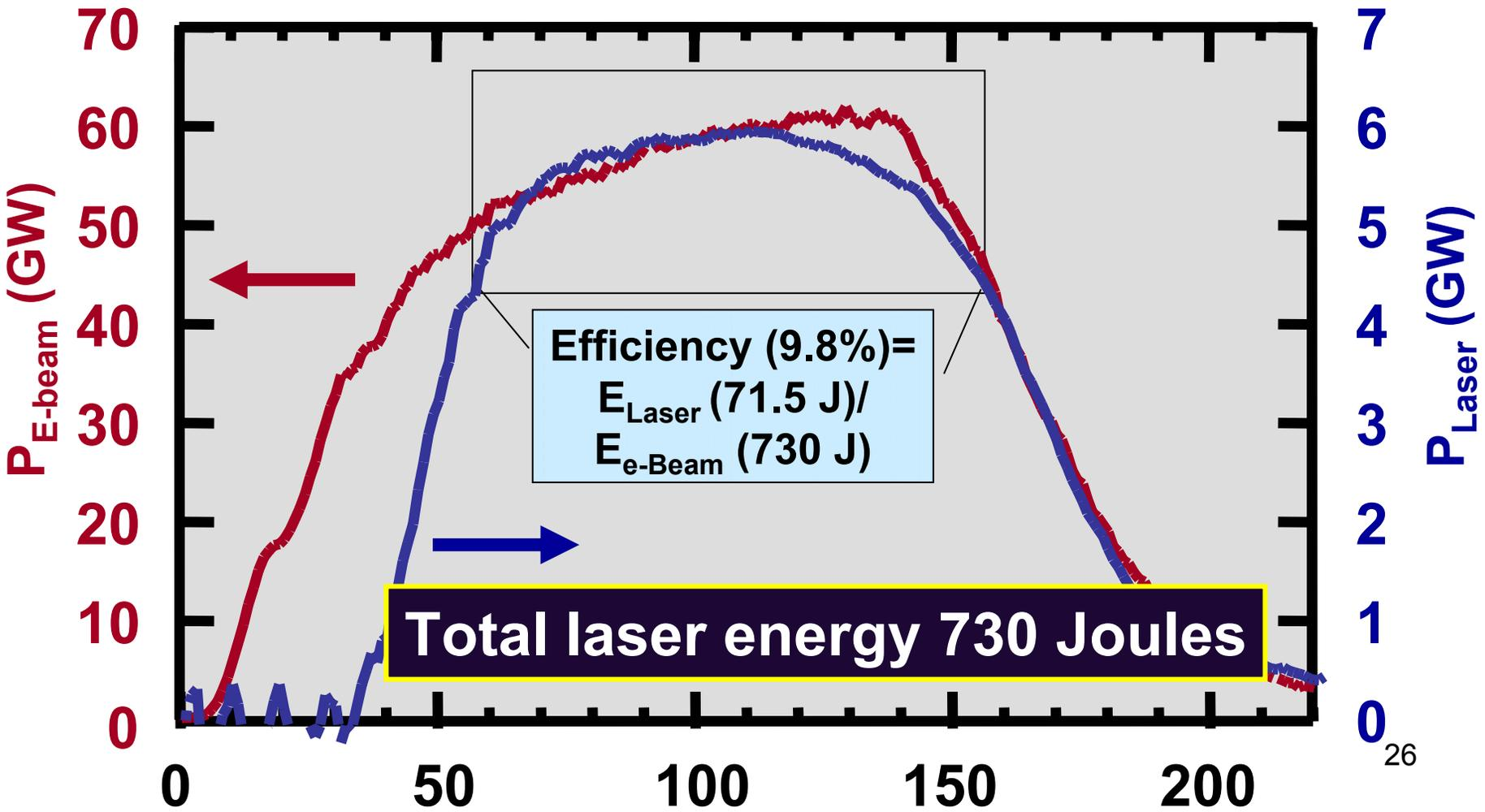
***Based on our research, an IFE-sized KrF system should have a wall plug efficiency > 7%***
