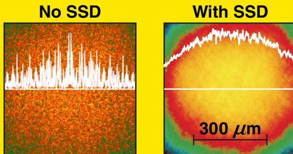
Verify laser imprint with foil-target experiments on OMEGA EP\*\*
