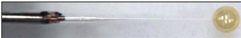
**Target: 2.95-mm OD, 20-μm wall**
