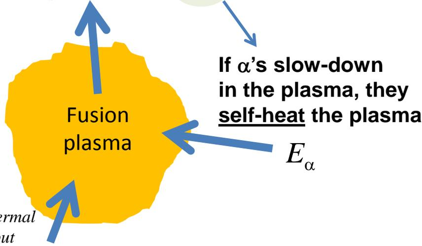
**External Thermal Energy Input to the Fusion Plasma**
