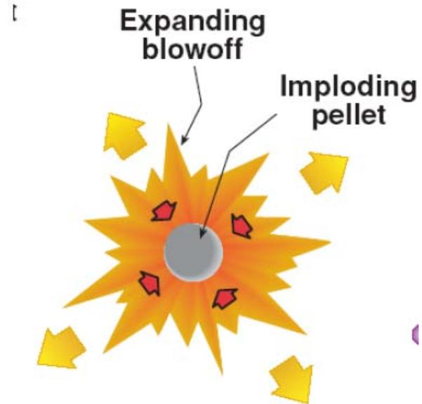
Implosion are driven by the rocket effect from the blow-off plasma.
