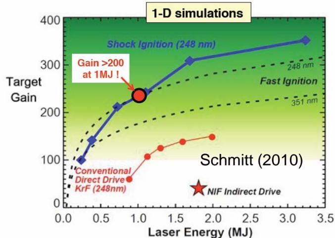
Shock Ignition uses hydrodynamic shocks to ignite the hot spot  $\rightarrow$  simple physics.
