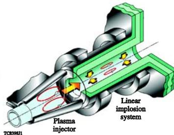
**Magnetized Target Fusion offers the potential for high wall-plug efficiency (but low target gains)**
