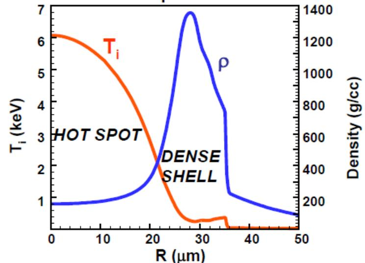
Ignition takes place in the “hot spot.” The thermonuclear instability (ignition) is triggered when the alpha self-heating exceeds all the energy losses in the hot spot
