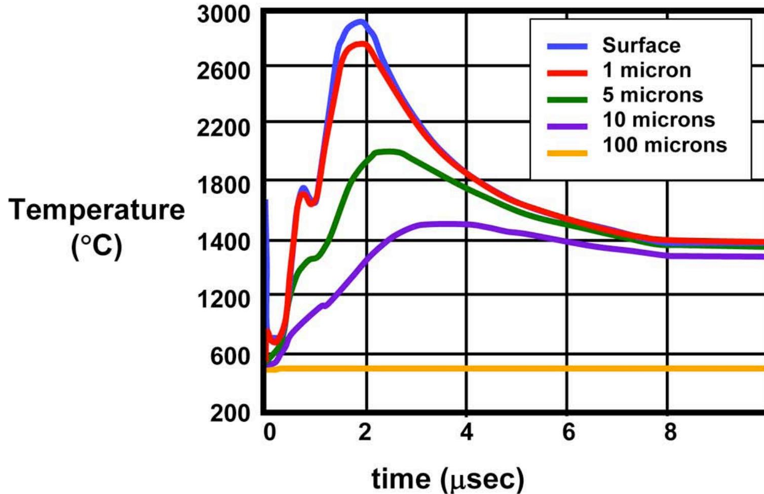
3 mm W armor, 154 MJ direct drive target spectra, 500 C coolant temperature
