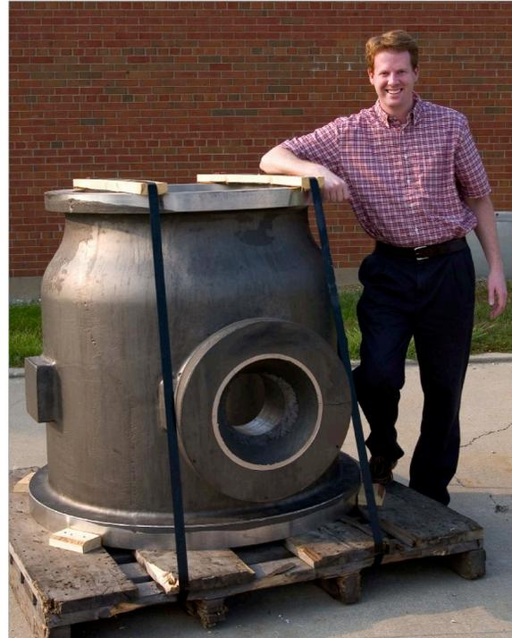
CF8C-Plus cast stainless steel: 10x improvement in thermal creep lifetime; 2 years from start of project to fabrication of components by industry
