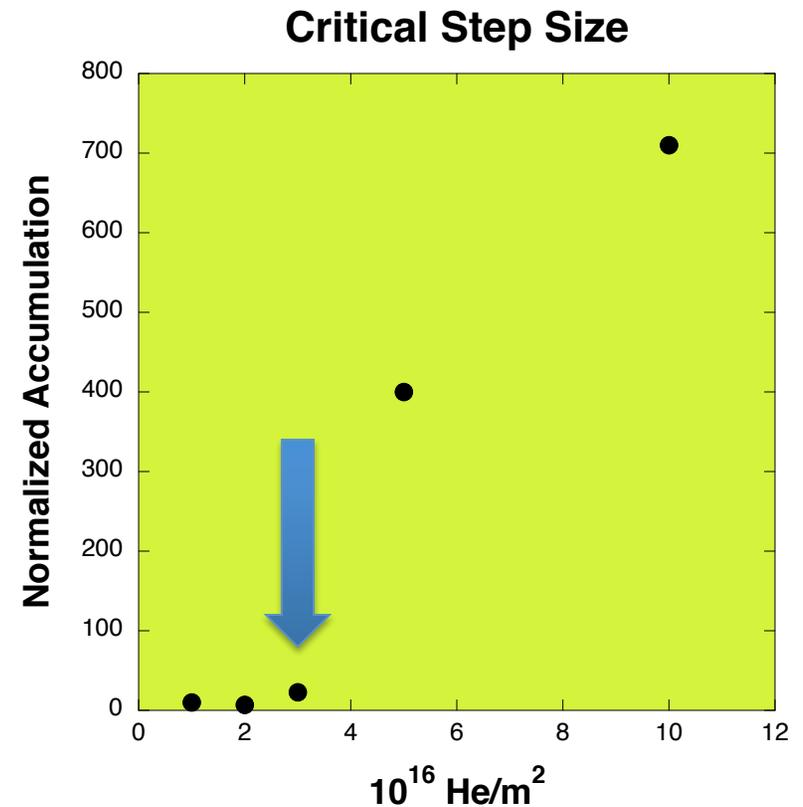
Retained He concentration is minimal if injected fluence prior to annealing is less than  $3 \times 10^{16} \text{ He/m}^2$  (for single crystal W)
