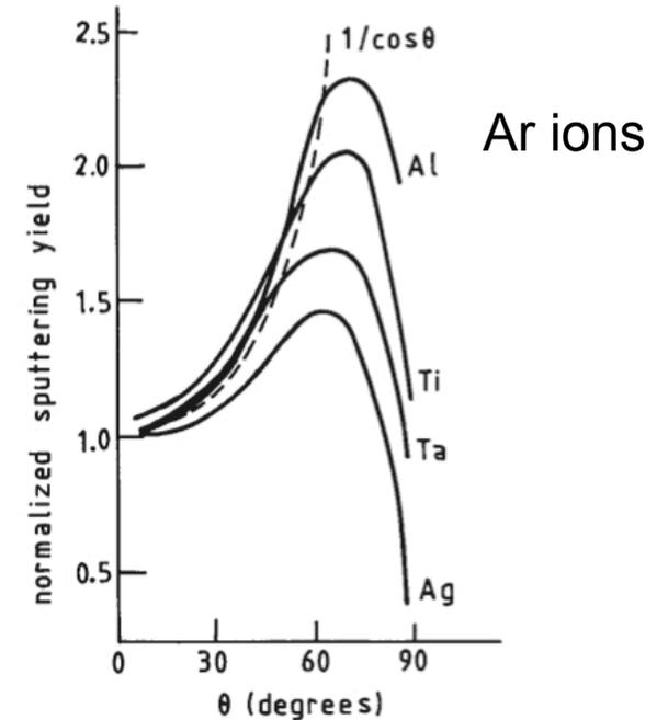
Figure 1. The sputtering yield, normalized to unity for ion incidence normal to the surface, as a function of the polar angle of incidence  $\theta$  with respect to the surface normal for 1.05 keV  $\text{Ar}^+$  ion bombardment of polycrystalline Al, Ti, Ta and Ag. (Adapted from
