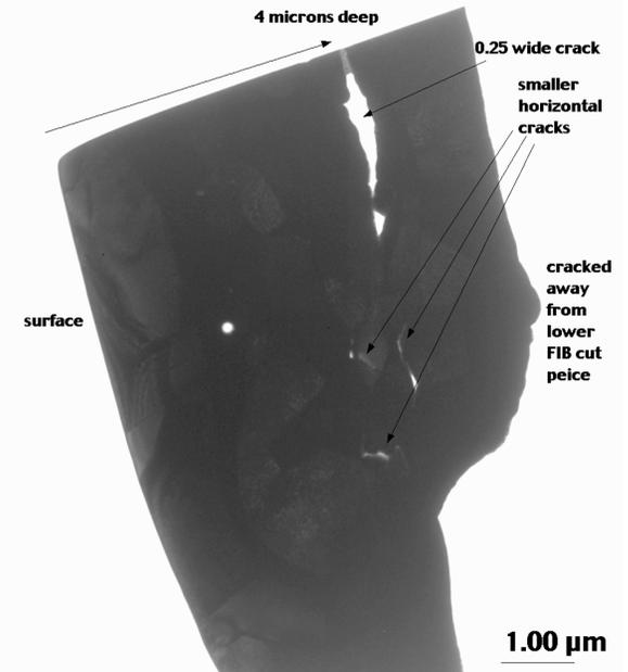
FIB/XTEM of 1000-pulse W, showing deep cracks evidently caused by fatigue, no surface melt
