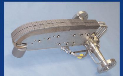
CfC monoblock and W brush armoured vertical target (EU).
