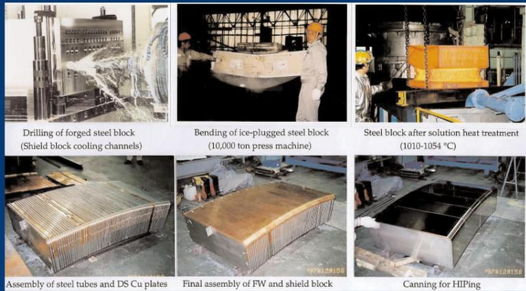
Full-scale prototype manufacture (JA).
