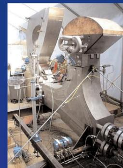
Inboard divertor channel integration mockup undergoing flow tests (US).
