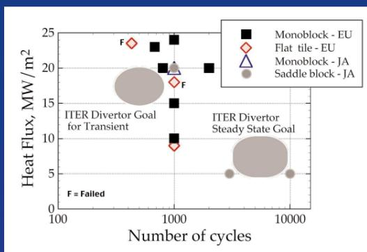
Results of CfC/Cu high heat flux component testing.
