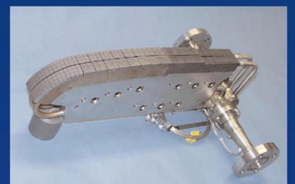
CfC monoblock and W brush armoured vertical target (EU).
