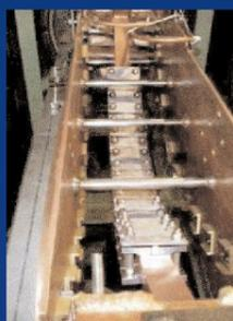
W and Be armour fast brazing to liner CuCrZr heat sink (RF).
