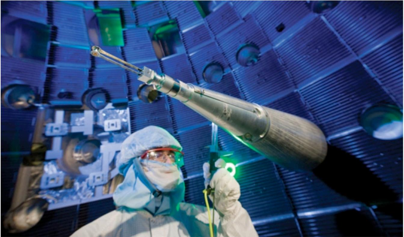
The NIF's lasers blast a tiny pellet containing isotopes of hydrogen to trigger fusion reactions.
