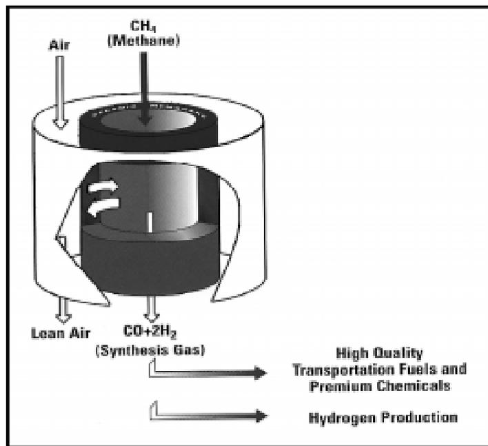
**Figure 4.3: The natural gas to liquids process.** Natural gas to liquids may be the process most nearly economical for making clean synthetic transportation liquids from fossil fuels other than oil. The cost can be reduced if oxygen can be extracted from air more efficiently than by cryogenic processing. DOE FE is supporting R&D on one promising method. It uses a high-temperature ceramic membrane to pass the oxygen as ions from the air side to the methane side.
