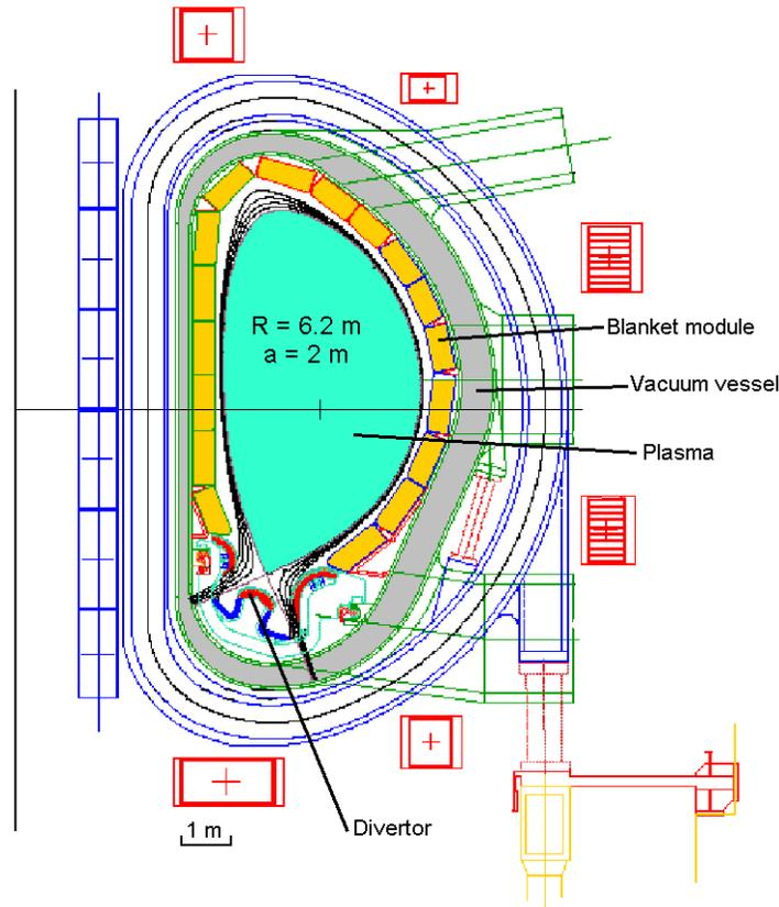
Figure 5 : ITER-Feat cross section
