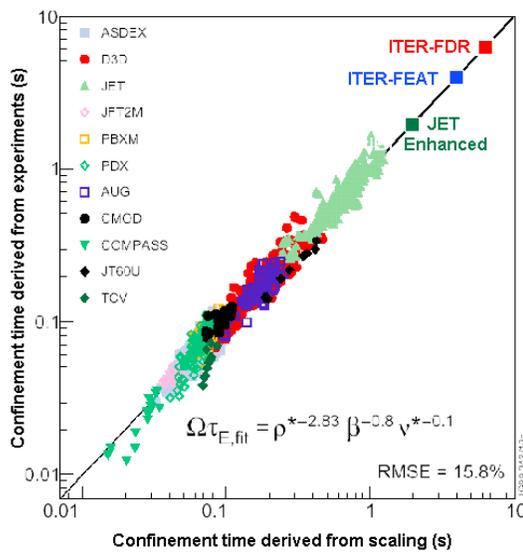
Figure 2 : Scaling law for energy confinement time
