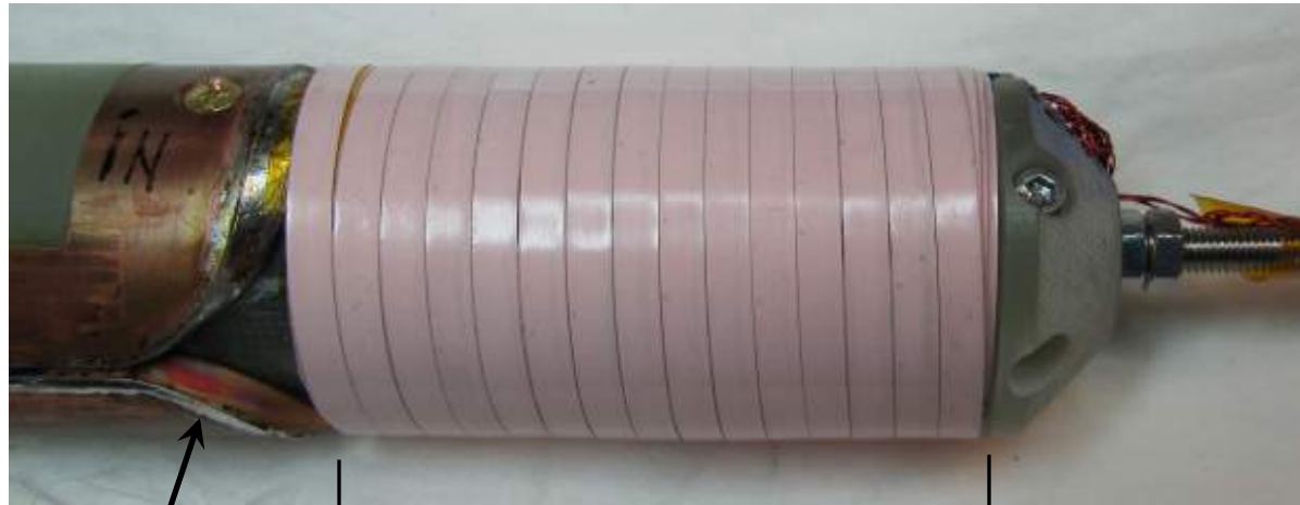
“Twist-bend” coil termination
